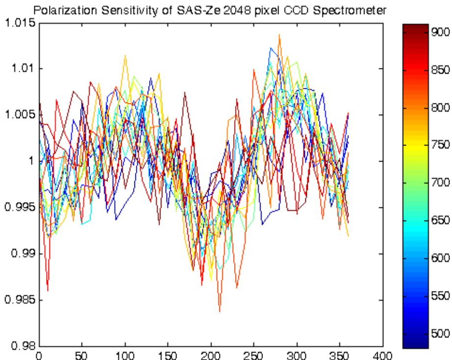
**Figure 12.** Polarization sensitivity of SASZe collector type "b" to 100% linearly polarized light.
