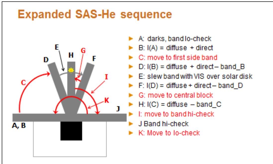
**Figure 10.** Expanded SASHe shadowband sequence with slew across solar disk (sequence E) to provide information on band alignment and the forward scattered lobe.
