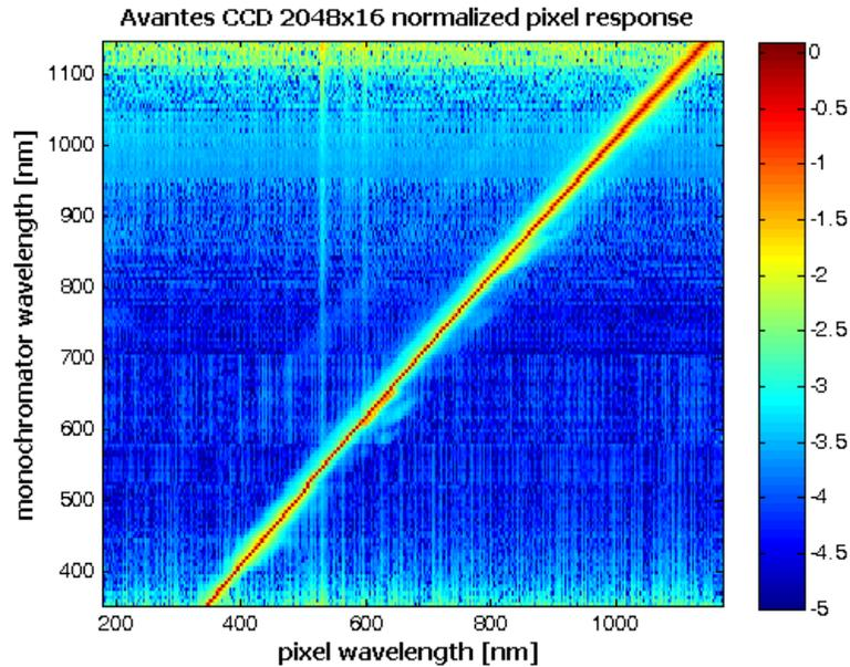
**Figure 11.** Example of spectrometer internal stray light measurement.
