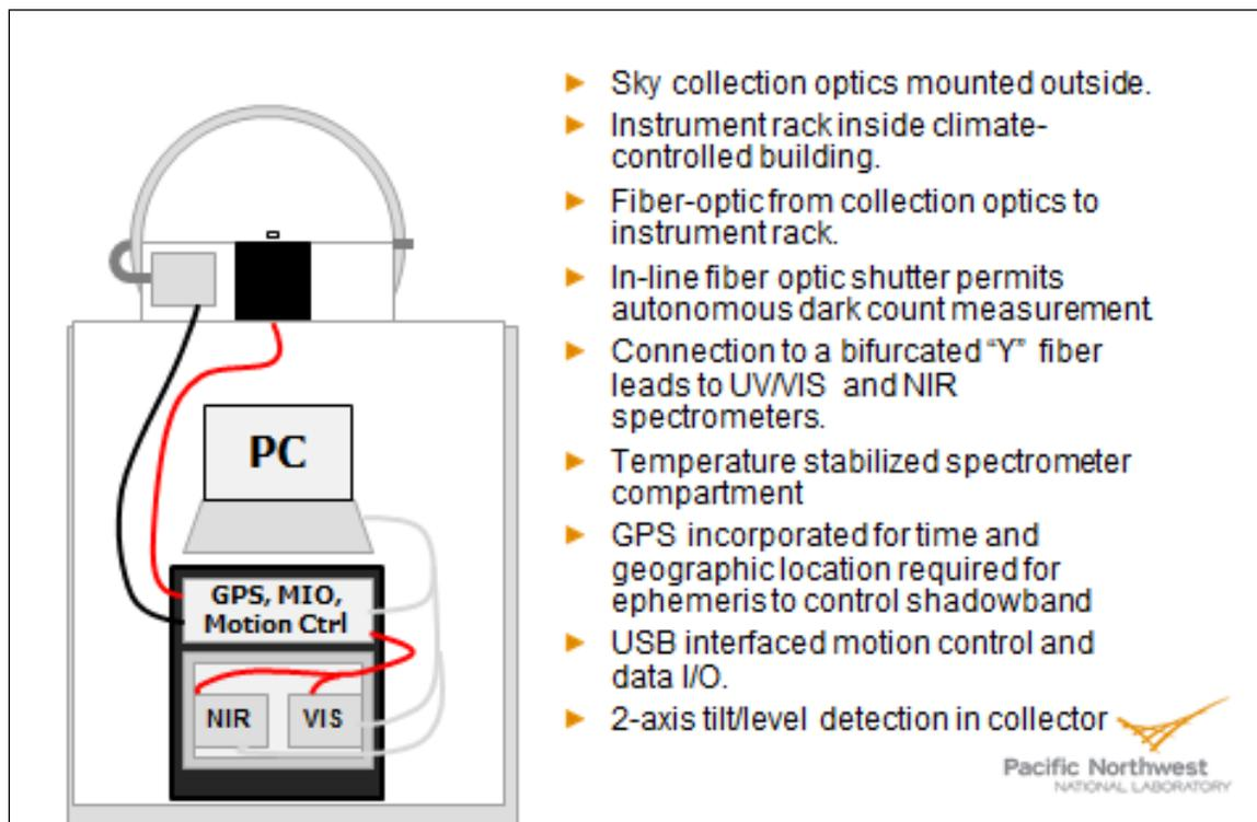
Figure 7. SAS instrument layout concept.
