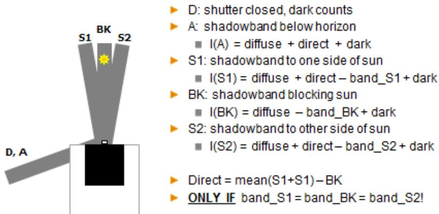
**Figure 9.** Basic SASHe shadowband sequence.
