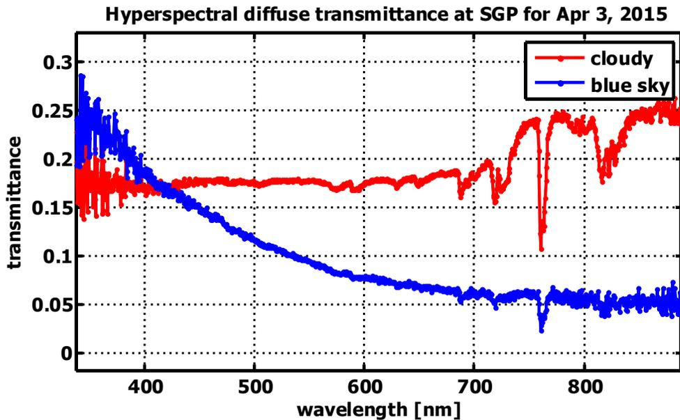
Figure 4. Clear sky (21 UT) and cloudy (16:30 UT) diffuse transmittance spectra exhibit sharply difference wavelength dependence.
