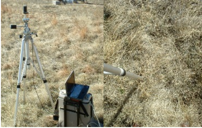
Fig. 7 Left: Deployment of an ASD field spectrometer at NREL in 2005. Right: Ground cover seen by the instrument in inverted position. (Photos courtesy Daryl Myers.)
