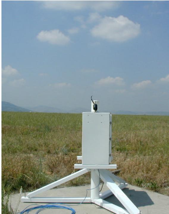
Figure 40. Side view of RSS, shown mounted on optional tripod.
