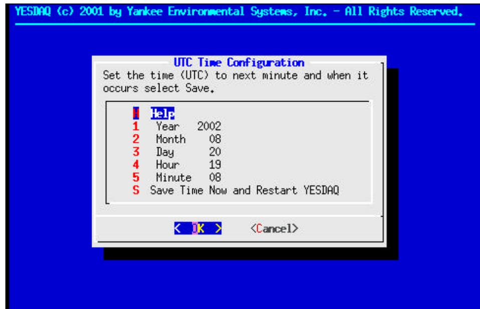
Figure 23. Main UTC Time Configuration Screen. If you setup time server, you do not need to set the time manually.
