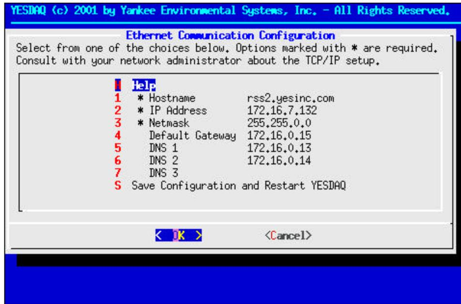
Figure 12. Main Ethernet configuration screen. NOTE: The settings shown here are for demonstration purposes only, DO NOT ENTER THESE SETTINGS! Instead, obtain a fixed TCP/IP address from your local network administrator.
