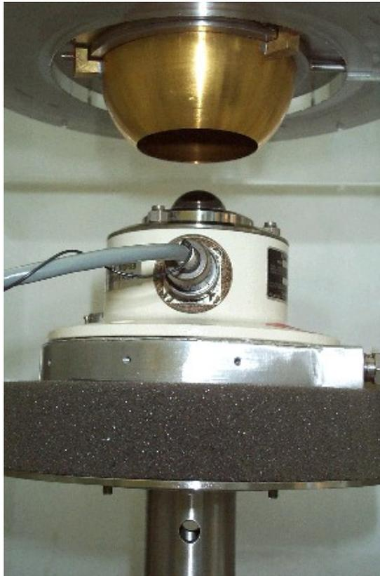
**Figure 5.** The PIR positioned below the PBCS completion hemisphere. During calibration, the PIR dome is fully inserted into the blackbody by means of the adjustable support mechanism.
