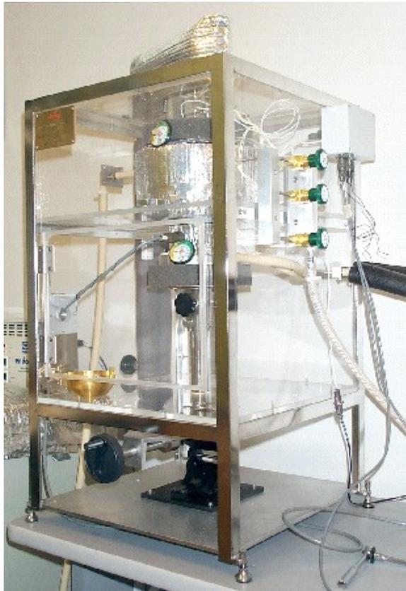
**Figure 4.** The calibration chamber portion of the Pyrometer Blackbody Calibration System.
