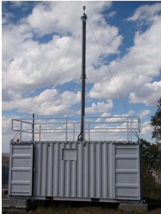
Figure 7. AOS instrument enclosure with 10-m sampling stack.
