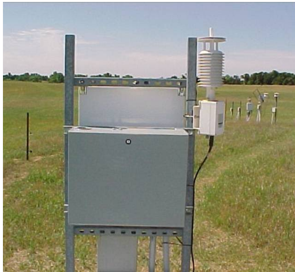
Figure 2. Infrared thermometer setup at the Southern Great Plains (SGP) observatory.
