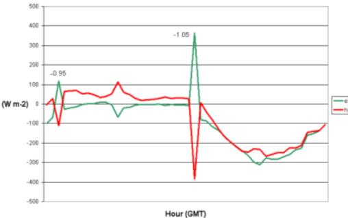
Figure 1. Plot showing sensible (h) and latent (e) heat fluxes showing a normal diurnal variation in heat fluxes. Spikes in the data occur at sunrise and sunset when the Bowen ratio is near -1.
