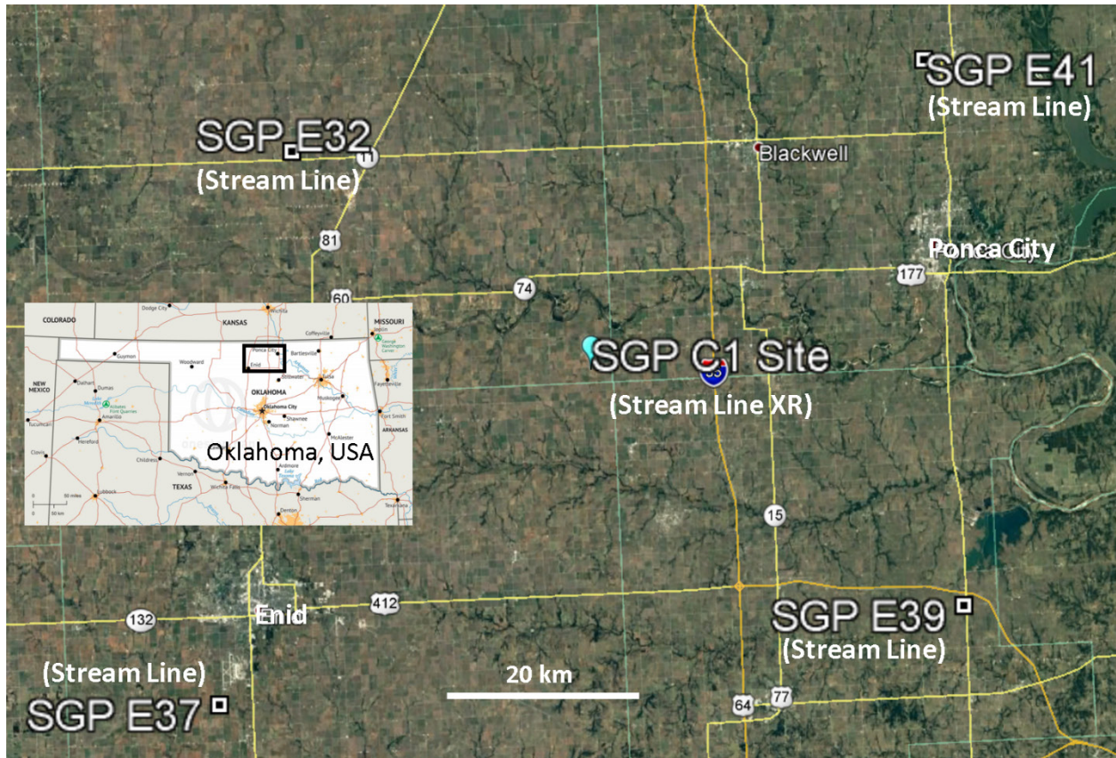
Figure 3. The network of five Doppler lidars at SGP includes one Halo Photonics Stream Line at each of the extended facilities (E32, E37, E39, and E41) and one XR and one XR+ at the Central Facility (C1).
