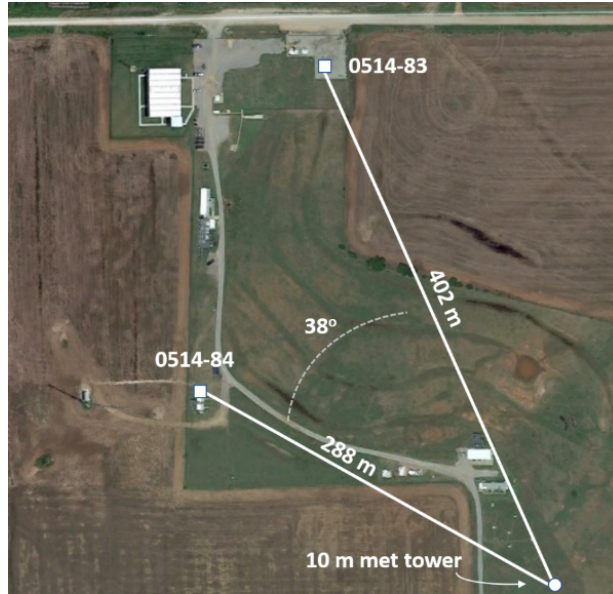
Figure 12. Instrument placement during the lidar-anemometer comparison test at SGP C1 in June 2014.
