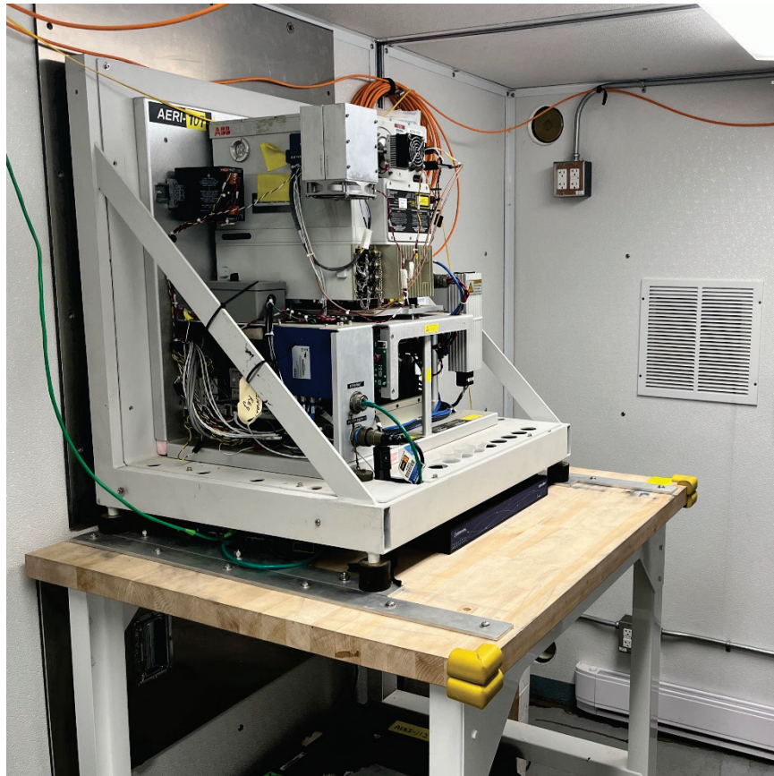
Figure 1. AERI back-end, in sea container in thru-wall configuration.
