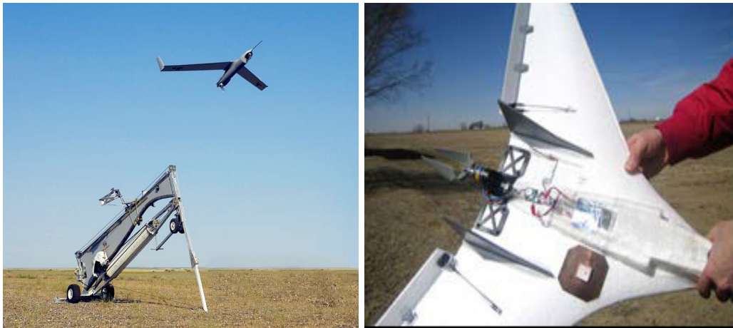
Figure 9. ScanEagle (left) and DataHawk (right) UAS, flown successfully at Oliktok during the “MIZOPEX” Campaign, July and August 2013.
