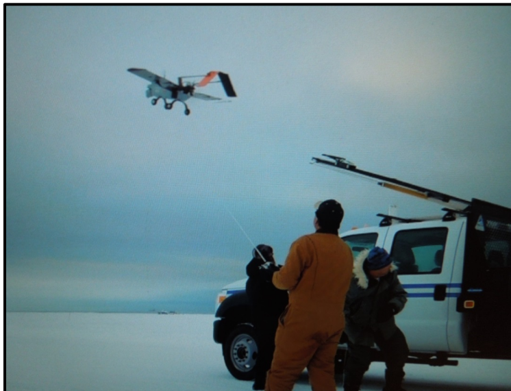
Figure 7. BAT-3 unmanned aircraft launched from a truck-mounted catapult located on the deactivated runway at the Oliktok Point Long-Range Radar Station.
