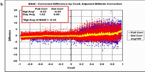
**Figure 10**. Residual differences between corrected PSP diffuse values and those from co-located Eppley 8-48 B&Ws for bi-mode (a) and adjusted bi-mode (b) methods for SGP data, by cosine of the SZA (CosZ). Blue is for Full correction, red for Detector Only correction. Yellow represents a 100-point running mean by CosZ through the data
