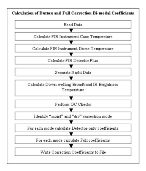
Figure 1. Flow diagram of nighttime fitting process.
