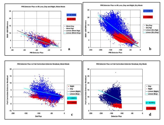
**Figure 9**. Day (blue) and night (red) relationships between the PIR detector flux, and the PSP IR loss (a, b), for the detector only correction moist mode (a) and dry mode (b). For the full correction (c, d), the residual difference after the PIR case-dome temperature portion of the correction has been applied for the moist (c) and dry (d) modes.
