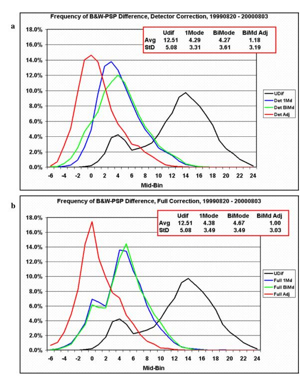
**Figure 12**. Frequency of residual differences between PSP diffuse measurements and co-located Eppley B&W for daylight (solar elevation greater than about 10°) corrections using detector only (a) and full (b) correction methodology. Black is for uncorrected PSP diffuse SW (Udif). Green is for single mode correction (1Md), blue is for bi-mode correction (BiMd). Red is for bi-mode adjusted correction (Adj).
