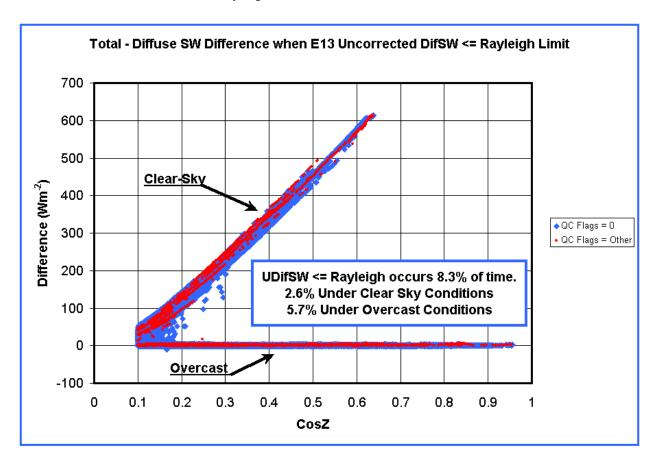
Figure 6. Difference between shaded and unshaded PSPs for sub-Rayleigh diffuse SW.
