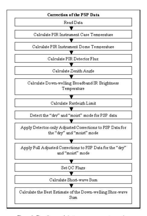
**Figure 4**. Flow diagram of shortwave measurement correction.
