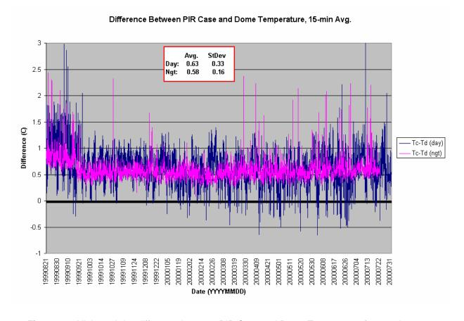
**Figure 14**. Night and day difference between PIR Case and Dome Temperature for 15-min average data.
