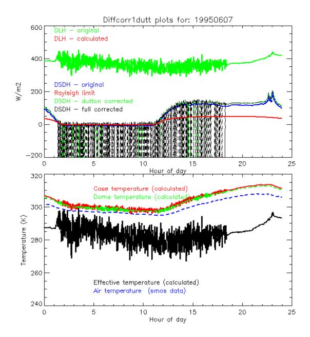
**Figure 16**. SIROS June 7, 1995, example of noisy pyrgeometer flux problem (green line, top plot) causing the majority of diffuse full corrected data to be rejected (black line, top plot). This noisiness is caused by noise in the case (red line, bottom plot) and/or dome (green line, bottom plot) temperature data. The corresponding ambient air temperature data (blue dashed line, bottom plot) shows that the rapid changes in case or dome temperature values are not real in nature.
