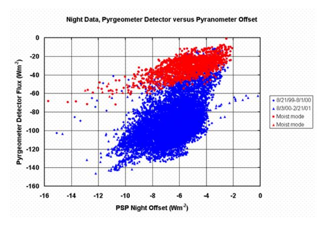
**Figure 2**. About 1.5 years worth of data from the ARM SGP Central Facility showing the PSP nighttime offset due to IR loss versus the corresponding PIR detector flux loss. Red points are those under "moist" conditions.
