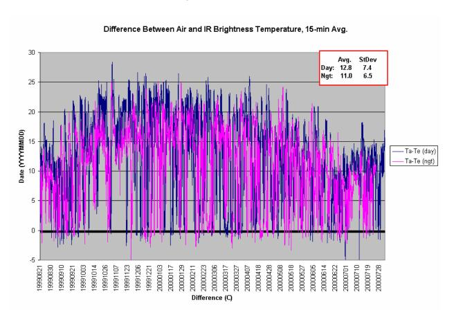
**Figure 15**. Night and day difference between Air and IR Brightness Temperature for 15-min average data.
