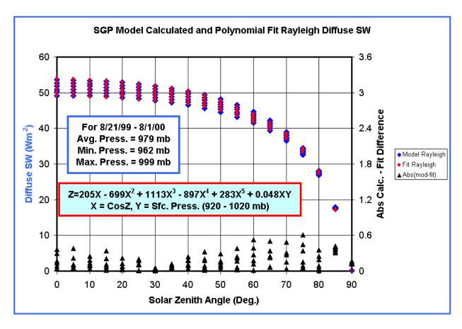
**Figure 5**. Model Rayleigh limit calculations for SGP (blue) and 5<sup>th</sup> order polynomial fit (red). Residual differences (black) are referenced to the right-hand axis.
