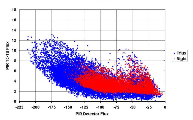
**Figure 3**. Relationship between PIR detector flux and the case-dome temperature term expressed as black body flux for the same data as that in Figure 2. Note that the relationship changes from uncorrelated to correlated at a detector flux of about -100 Wm<sup>-2</sup>. Also note the greater occurrence of larger detector flux loss during day than at night
