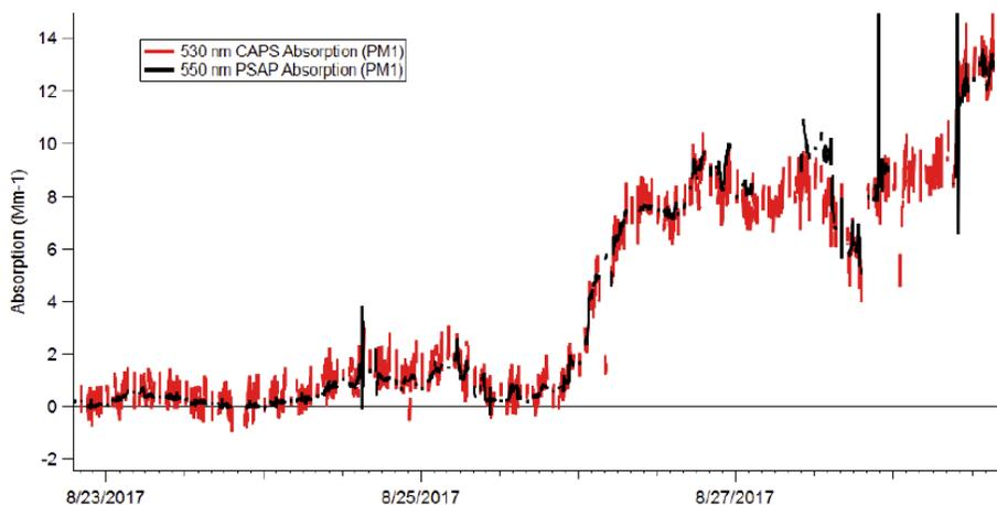
**Figure 13.** Cavity-attenuated phase shift (CAPS) and particle soot absorption photometer (PSAP) aerosol light absorption measurements for late August, 2016, Ascension Island. Plot courtesy of Tim Onasch.
