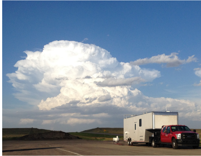
Figure 2. The University of Wisconsin-Madison SPARC facility, which was designated mobile PISA #3, during PECAN. The ARM Doppler lidar is shown deployed on the surface beside the trailer. The SPARC facility included an AERI and a High Spectral Resolution Lidar (HSRL) on board, and was able to launch radiosondes.
