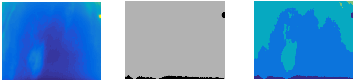
Figure 2. ICI images from Barrow: radiance in \text{W m}^{-2} \text{sr}^{-1} (left), conventional binary cloud map showing cloudy and clear pixels (center), and cloud map showing upper-limit cloud optical depth (right).
