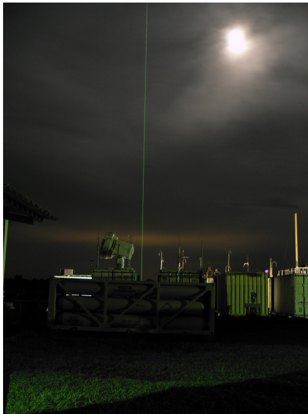
Figure 2. The green laser beam of the mobile Raman lidar from IPEN-USP, our reference system, taking measurements at the ARM site in Manacapuru. Photo by Rebecca Wernis.
