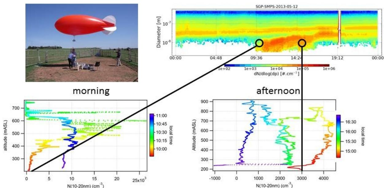
**Figure 4.** Tethered balloon data showing vertically resolved data on 10-20 nm diameter particle number concentrations during the NPFS.
