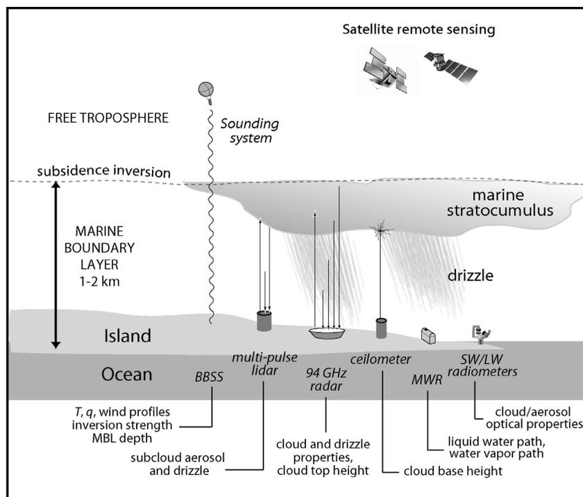
**Figure 7.** Schematic showing key instruments to be used in the AMF deployment.
