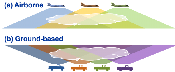
Fig 1. Schematic of two mobile cloud tomography setups. The swath of each radiometer scan cycle is shown in different color.
