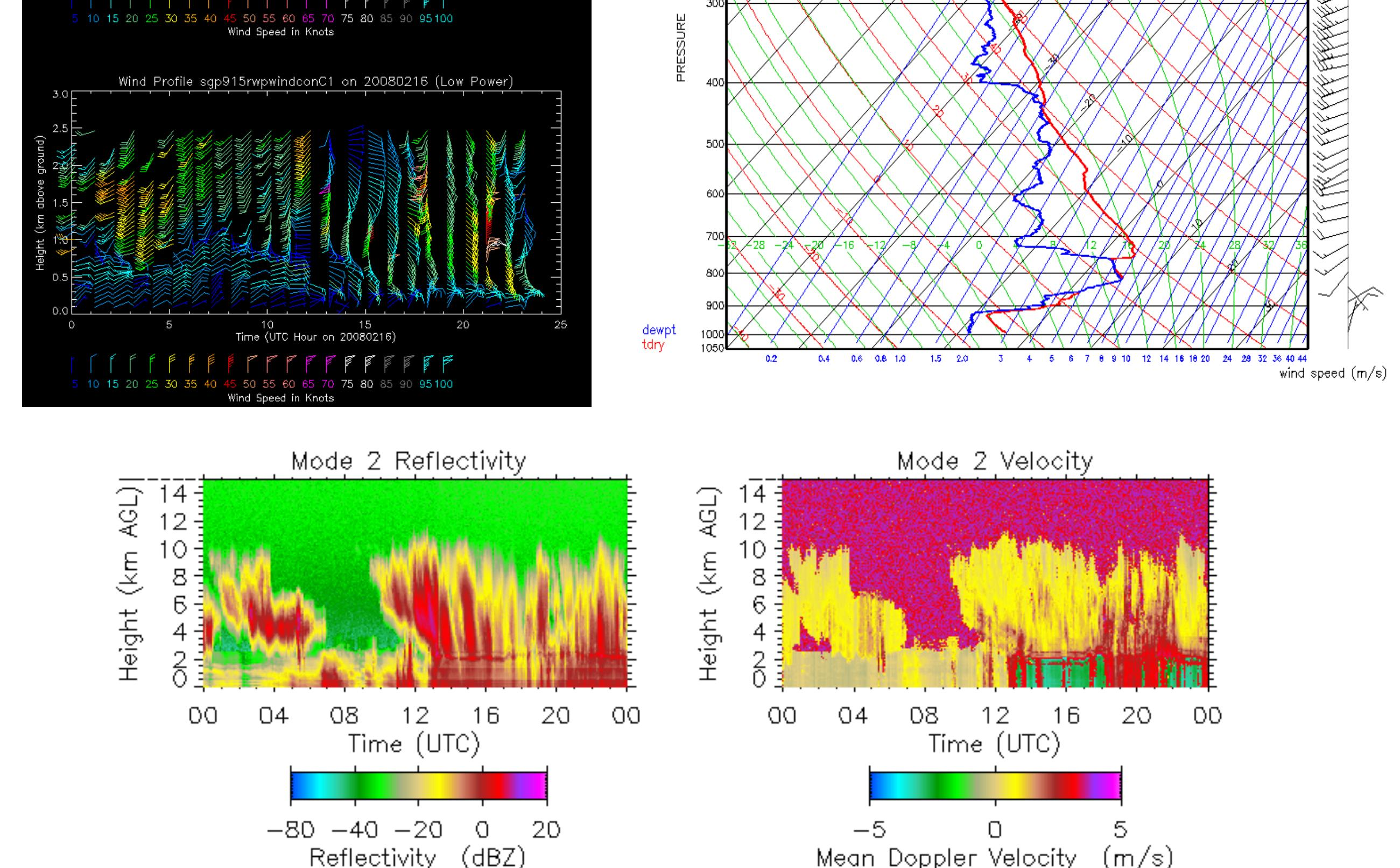
MMCR data from the SGP Central Facility clearly show small scale details that can be used to diagnose microphysical quantities. Such calculations will be even more valuable when coupled with W-band (WACR) data.
