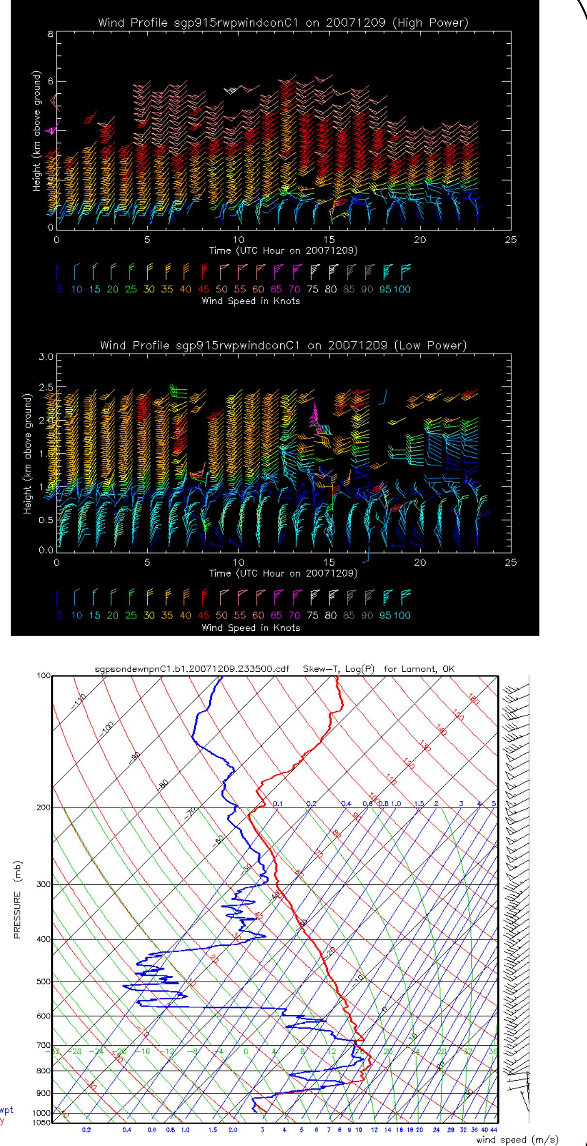
The SGP's 915 MHz profiler winds clearly show the cold layer at the surface dominated by northerly winds. Continued cold advection during the 9<sup>th</sup> deepened the layer.
