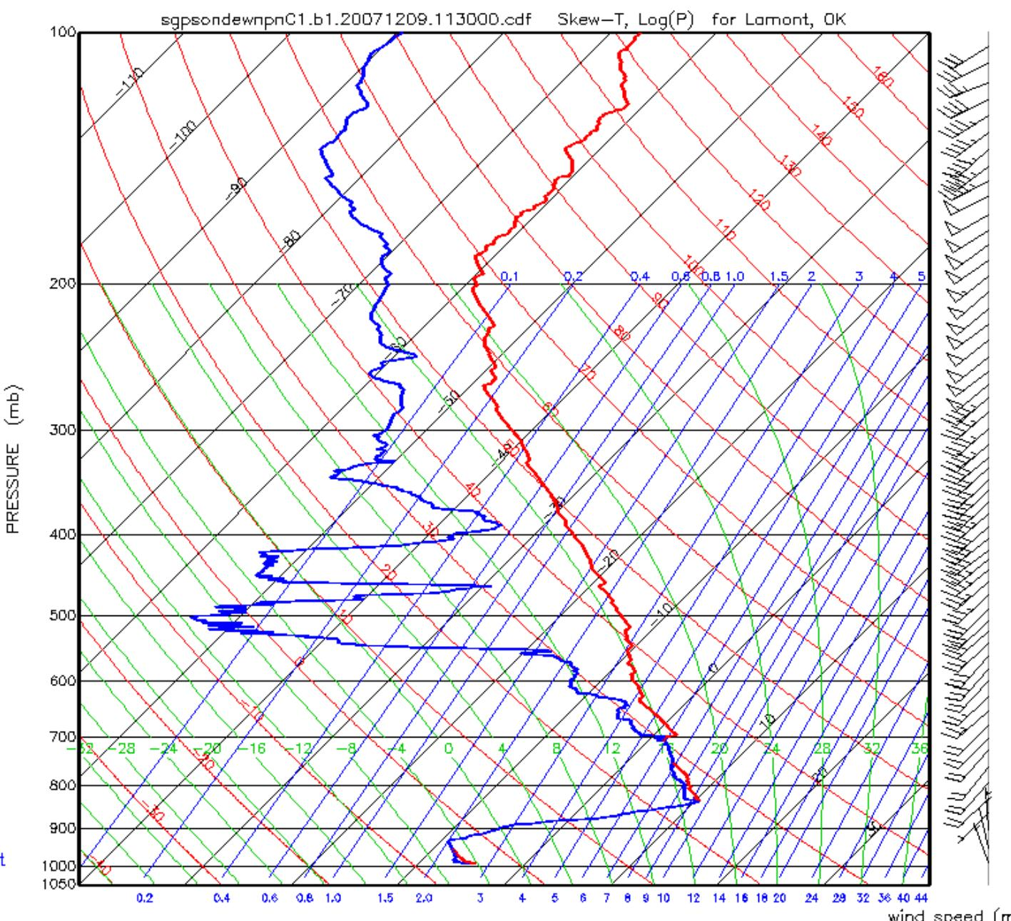
The SGP's 1130 UTC sounding on the 9th clearly shows the cold air at the surface (-5°C) and very warm air just above the surface (10°C and saturated at 830 mb). The storm system tapped instability in the air above 850 mb to cause convective cells that contributed to much of Oklahoma's heavy icing.
