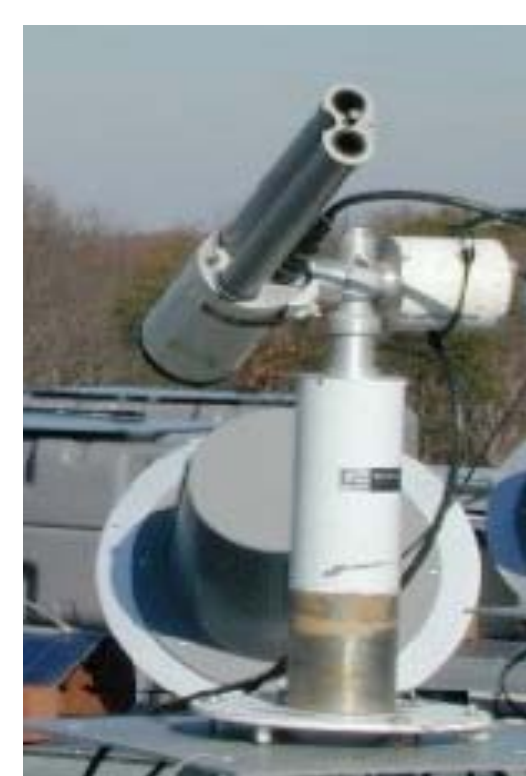
Cimel Normal aerosol mode (sun-seeking)
