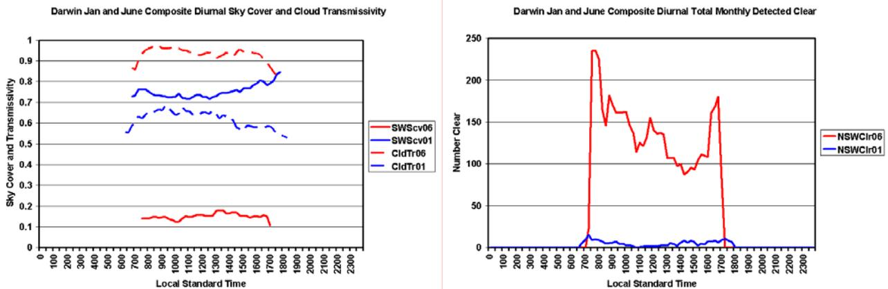
**Figure 5.** Left: Composite average monthly diurnal daylight fractional sky cover (solid) and cloud field effective transmissivity (dashed) for January (blue) and June (red). Right: Same as left but for the number of daylight 1-minute data detected as clear-sky for Jan. (blue) and June (red).
