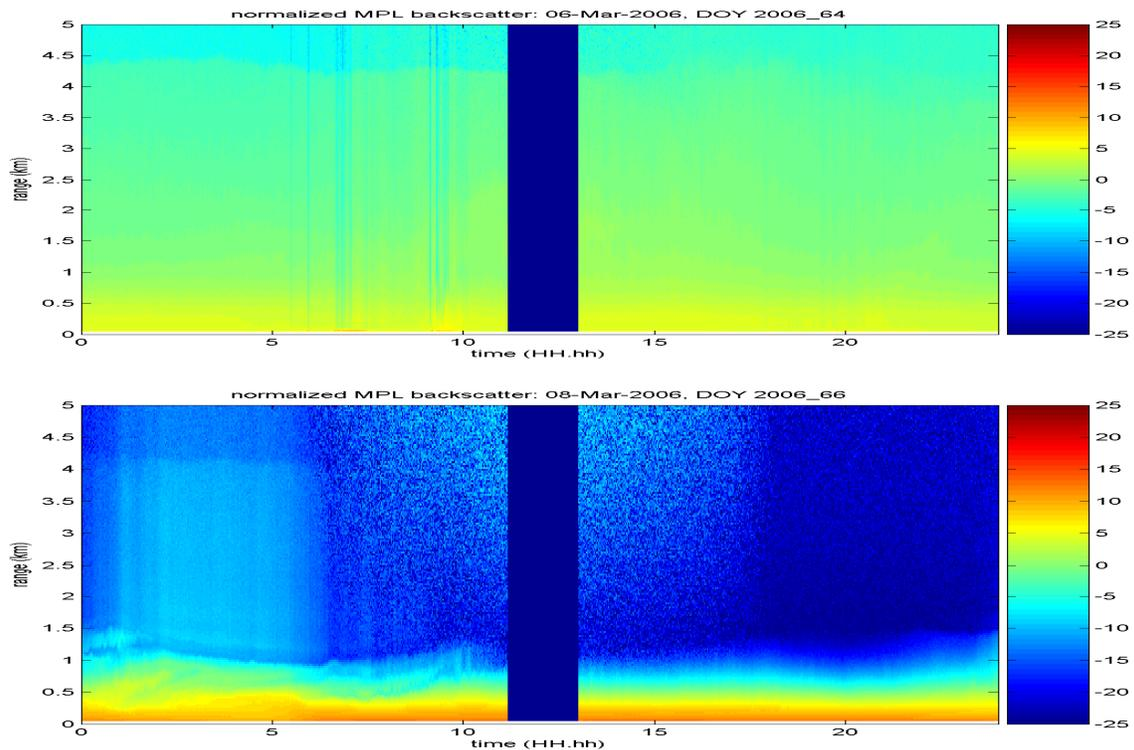
**Figure 2.** Examples of normalized MPL backscatter for clean day (top) and dust storm (bottom).
