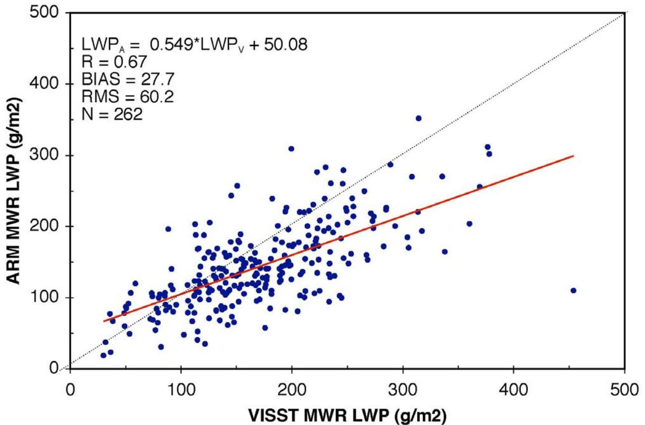
Figure 6. Comparison of VISST and MWR derived liquid water path.
