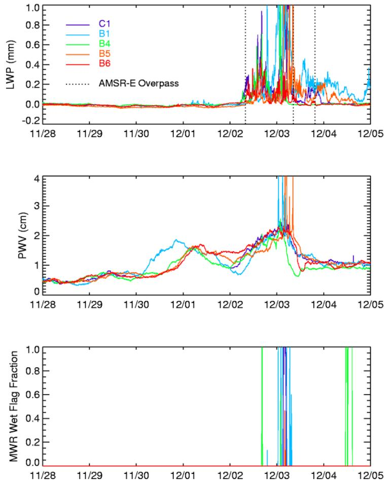
**Figure 2.** Time series of LWP, PWV, and wet-flag fraction recorded by five ground-based microwave radiometers at the ACRF SGP site between November 28 and December 5, 2003. AMSR-E overpass times on December 2 and 3 are indicated by vertical dotted lines in top panel.
