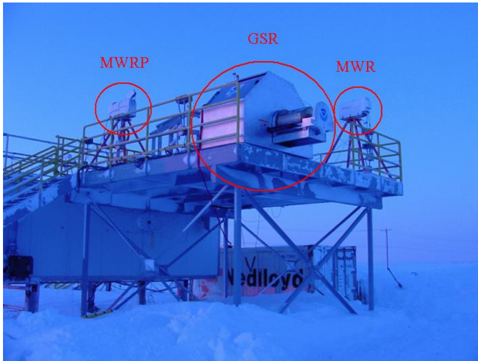
Figure 3. The experimental set-up on the skydeck during the 2004 Water Vapor IOP. The GSR was located by the operational ARM MWRs, the MWR, and the MWE profiler (MWRP).
