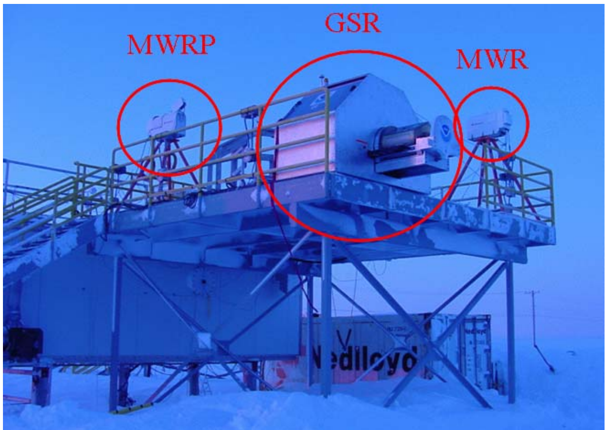
Figure 1. Photo of the GSR, ARM MWR, and the ARM MWPR at the NSA/AAO Great White site near Barrow, Alaska.
