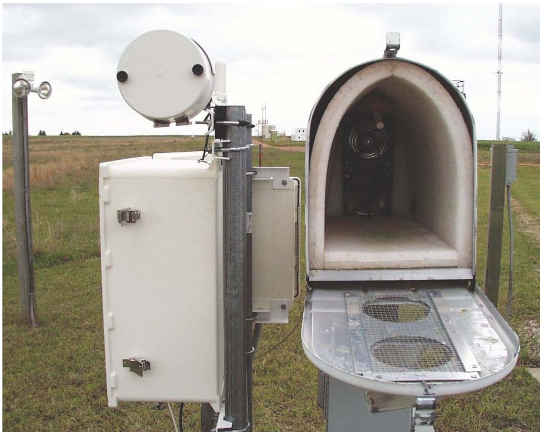
Figure 1. Prior to launch, radiosondes are placed in this ventilated mailbox at the SGP radiosonde launch site. The mailbox contains a Rotronic T/RH sensor and the sampling inlet for a chilled-mirror hygrometer that is located in the box at left. Additional T/RH measurements outside the mailbox are made by the THWAPS sensors in the round housing.
