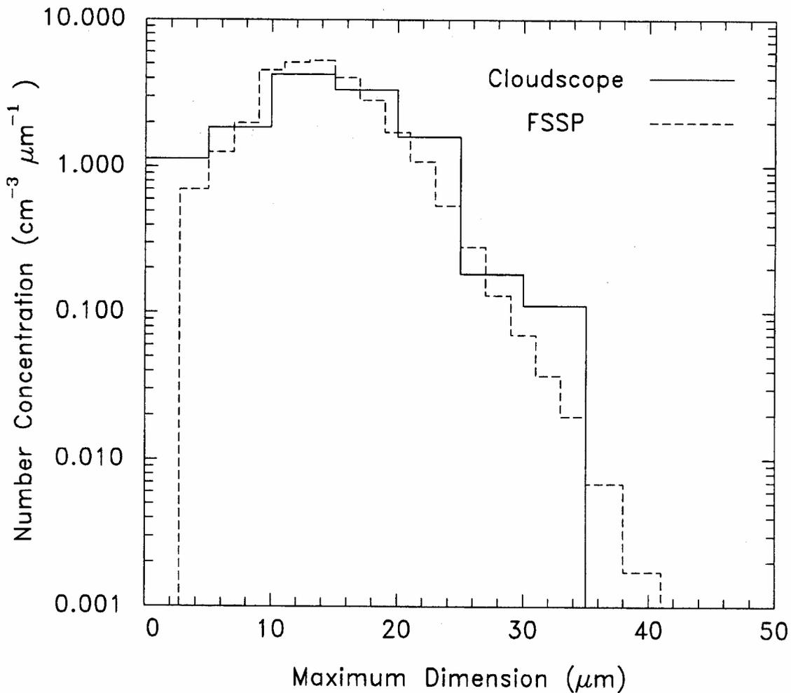
**Figure 1.** Comparison of size spectra measured by the CS and FSSP for hexagonal columns in a laboratory grown ice cloud.
