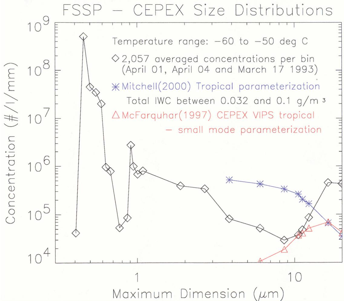
**Figure 3.** Comparison of FSSP - CEPEX SD (in black), plotted together with Mitchell (2000) tropical parameterization (in blue) and McFarquhar (1997) CEPEX VIPS tropical small mode parameterization (in red).
