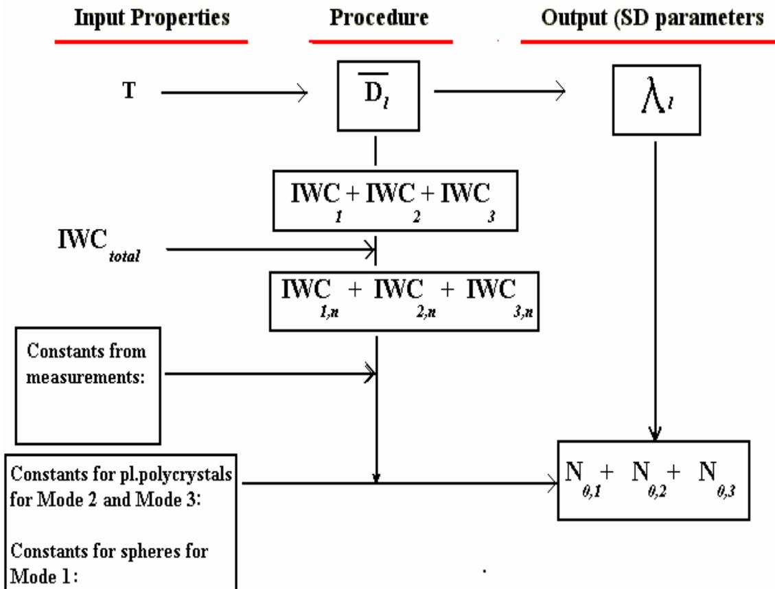
**Figure 8.** Flow chart describing the methodology used to parameterize tropical trimodal size spectra. Note: Planar polycrystals are assumed for the shape of Mode 2 and Mode 3 ice crystals and spheres are assumed for the very small Mode 1 crystals. This methodology illustrates the procedure for acquiring all nine of the gamma parameters for trimodal size spectra. SD constant values were obtained directly from measurements and are listed in Table 1.
