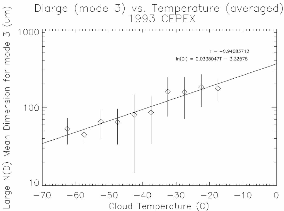
**Figure 7.** Mean dimension measured by the 2DC vs. temperature for this study (CEPEX). Vertical bars are standard deviations. Note the high correlation coefficient  $r = -0.9408$ .
