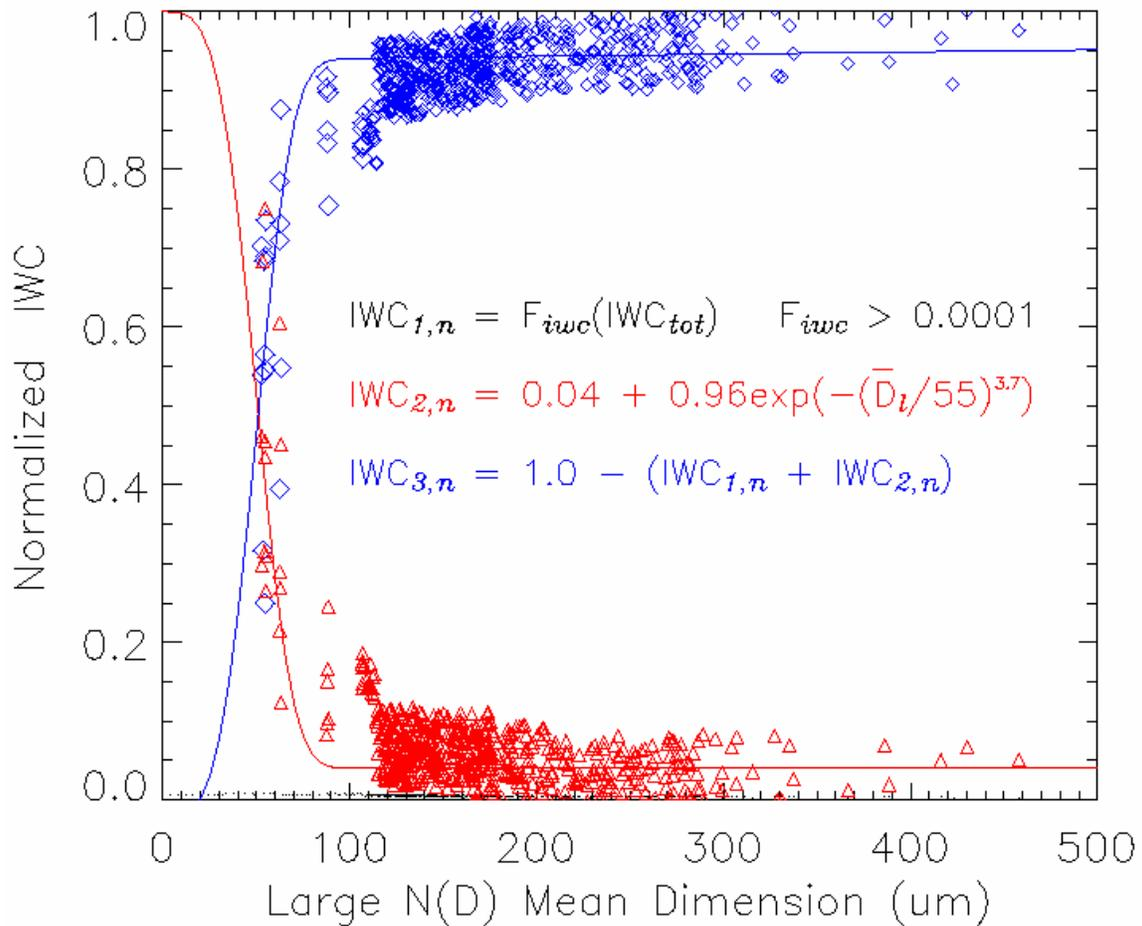
**Figure 9.** Normalized IWC calculated from the FSSP and 2DC related to the large mode (Mode 3) mean size  $D$ .
