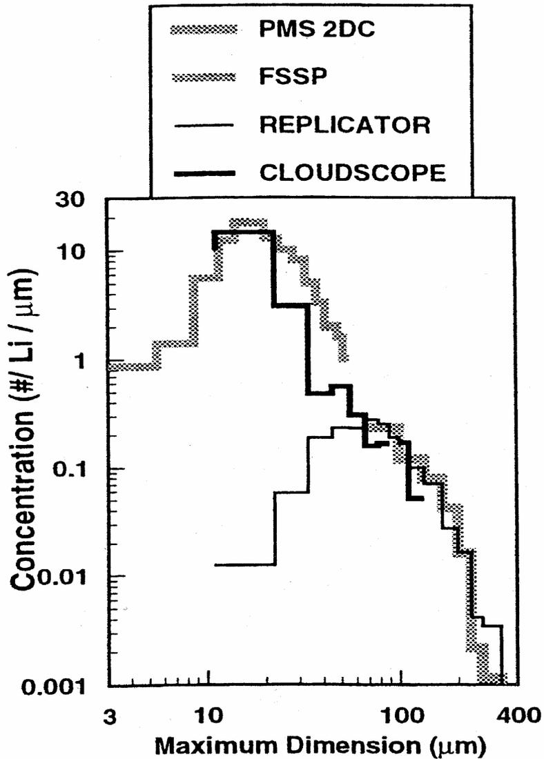
**Figure 2.** Size spectra from September 26, 1997, U.S. Department of Energy (DOE)-ARM Program IOP, Hurricane Nora outflow, 19:09:15 - 19:11:00 Universal Time Coordinates,  $-48.3^{\circ}\text{C}$  to  $-50.3^{\circ}\text{C}$ , 11.95 km to 12.18 km, T.A.S. = 118.5 m/s.
