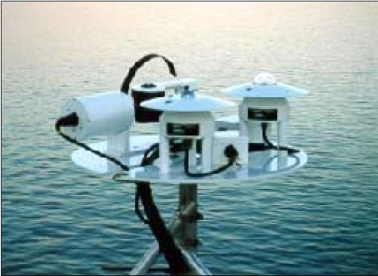
**Figure 1.** The portable radiation package with its FRSR.
