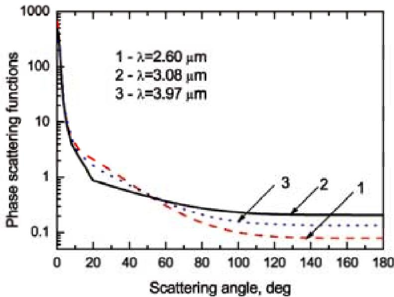
**Figure 1.** Scattering phase functions for wavelengths  $\lambda = 2.60 \mu\text{m}$ ,  $\lambda = 3.08 \mu\text{m}$ , and  $\lambda = 3.97 \mu\text{m}$ . Calculations are made for systems of ice plates and columns by the method of Petrushin (1998).
