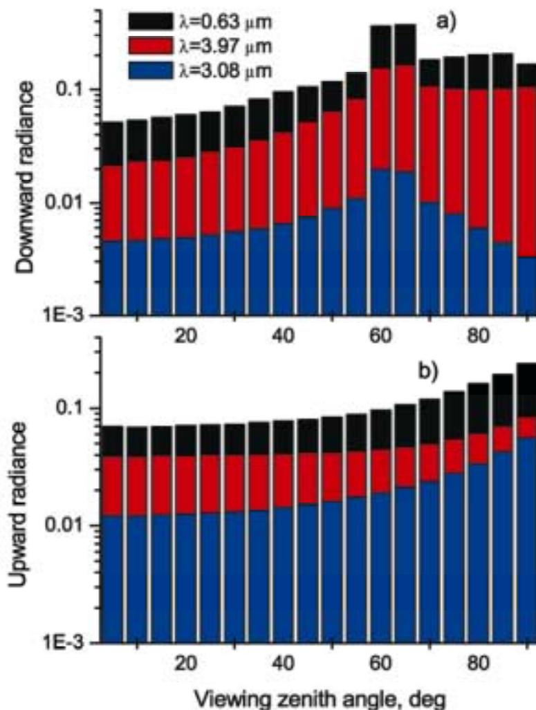
**Figure 4.** Angular distributions of solar radiation for different wavelengths in 3D cloud model. Calculations are made for optical depth  $\tau = 1$ ; solar zenith angle  $\xi_{\oplus} = 60^\circ$ ; cloud fraction  $N = 0.5$ ;  $D_x = 2 \text{ km}$ ,  $D_y = 100 \text{ km}$ ; and surface albedo  $A_s = 0.2$ .
