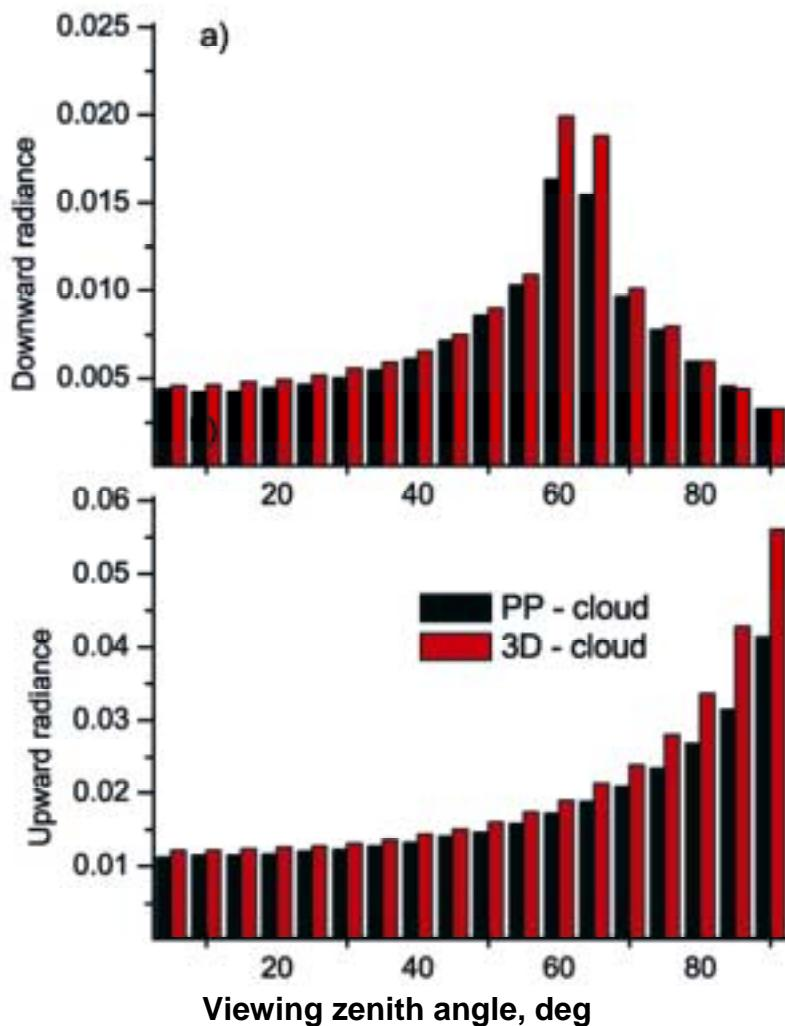
**Figure 3.** Angular distributions of solar radiation calculated with (3D-cloud) and without (PP-cloud) account of random cloud geometry for wavelength  $\lambda = 3.08\mu\text{m}$ ; optical depth  $\tau = 1$ ; solar zenith angle  $\xi_{\oplus} = 60^\circ$ ; cloud fraction  $N = 0.5$ ; and surface albedo  $A_s = 0.2$ .
