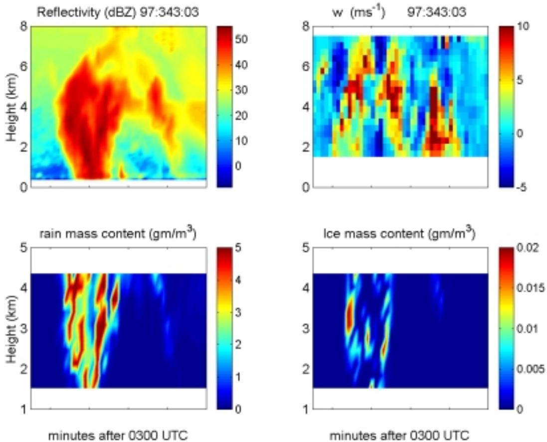
**Figure 1.** Time height cross sections of radar reflectivity, vertical motion, rain water content, and hail mass content measured using two wind profilers in Darwin, northern Australia, as a shallow thunder storm passed over the observing site. The rain is derived using the reflectivity-weighted fall speed spectrum. The hail is estimated using the spectral information at velocities in excess of the asymptotic limit for rain.
