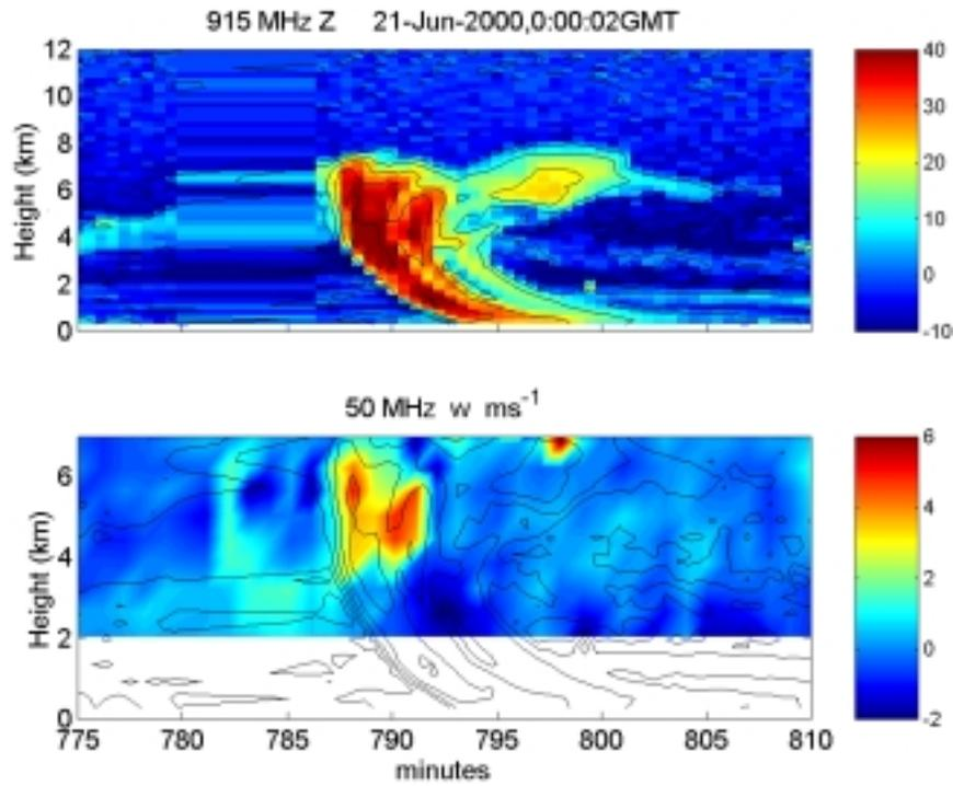
**Figure 2.** Time height cross sections are radar echo power and vertical motion of an isolated thunderstorm that passed over the CART site in Northern Oklahoma.
