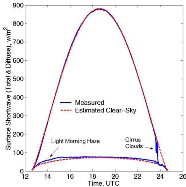
**Figure 6.** Measurements and estimated clear-sky values (calculated via Chuck Long's technique) for the total and diffuse surface shortwave flux on March 20, 2000.
