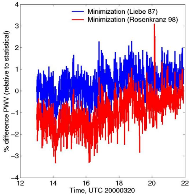
**Figure 7.** Relative difference between the statistical approach and the minimization approach using the Liebe 87 (blue line) and Rosenkranz 98 (red line) for March 20, 2000.
