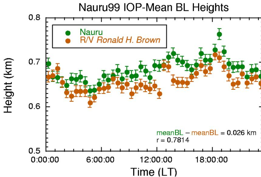
**Figure 5.** The mean daily cycle of BL heights over Nauru and the R/V *Ronald H. Brown* during the Nauru99 IOP. Error bars indicate the standard error of each value.
