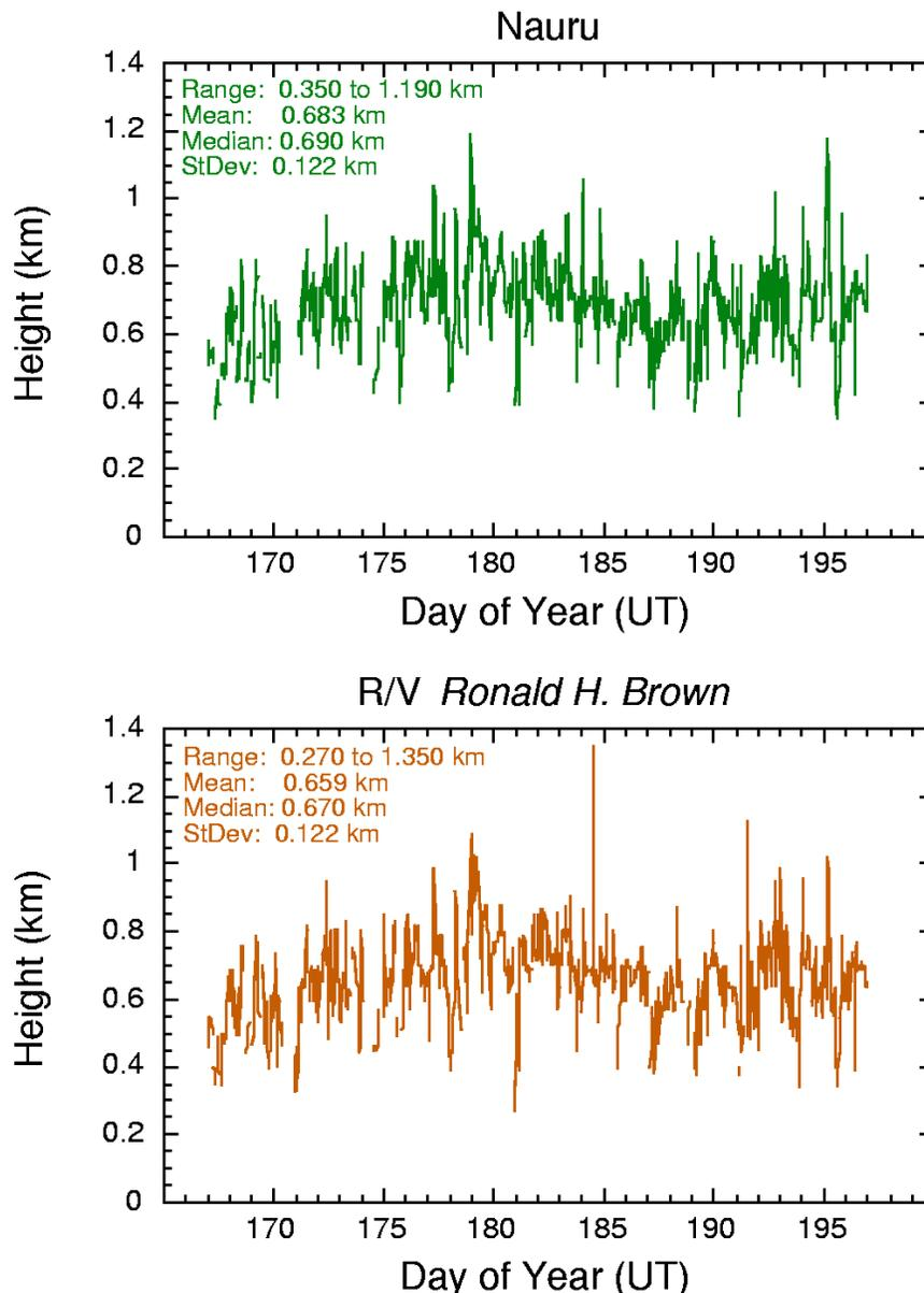
**Figure 4.** The height of the atmospheric boundary layer over Nauru (top) and the R/V *Ronald H. Brown* (bottom) during the Nauru99 IOP.
