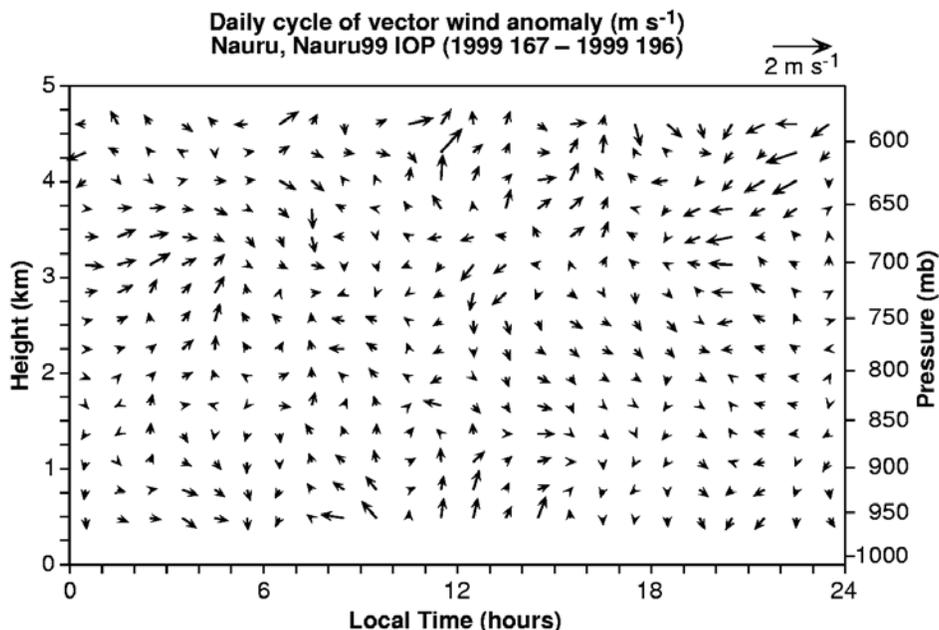
**Figure 2.** The daily cycle of vector wind anomalies at Nauru during the Nauru99 IOP (June 16 through July 15, 1999) as a function of height (or pressure). Arrow sizes are proportional to speed; a  $2 \text{ m s}^{-1}$  reference vector is shown above the upper right-hand corner.
