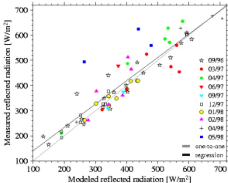
**Figure 5.** Comparison of the measured reflected broadband shortwave radiation (GOES-8 satellite) and the modeled reflected shortwave radiation at TOA.
