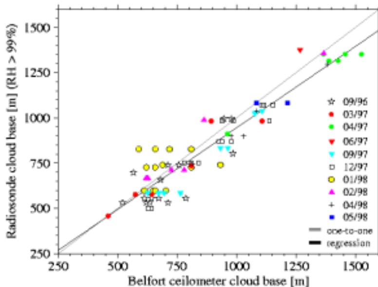
**Figure 4.** Comparison of the height of the cloud base measured with the ceilometer and during a radiosonde ascent (criterion: relative humidity exceeds 99%). Both measurements indicate the height above mean sea level (the ARM SGP site lies at 315m).
