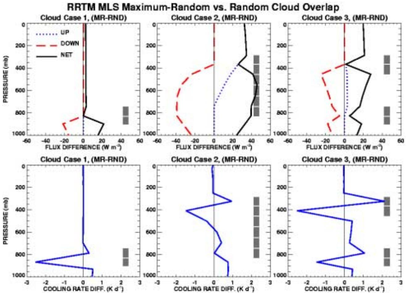
**Figure 2.** Differences in longwave up, down, and net fluxes (top row) and cooling rates (bottom row) between MR cloud overlap and random overlap as calculated by RRTM for three cloud cases. Layers with cloud are marked with gray boxes to the right in each plot. All clouds have an optical depth of 5 in each layer. Cloud cases 1 and 2 are for cloud fractions of 1.0 on each layer, and cloud case 3 has cloud fractions of 0.5 in each layer.
