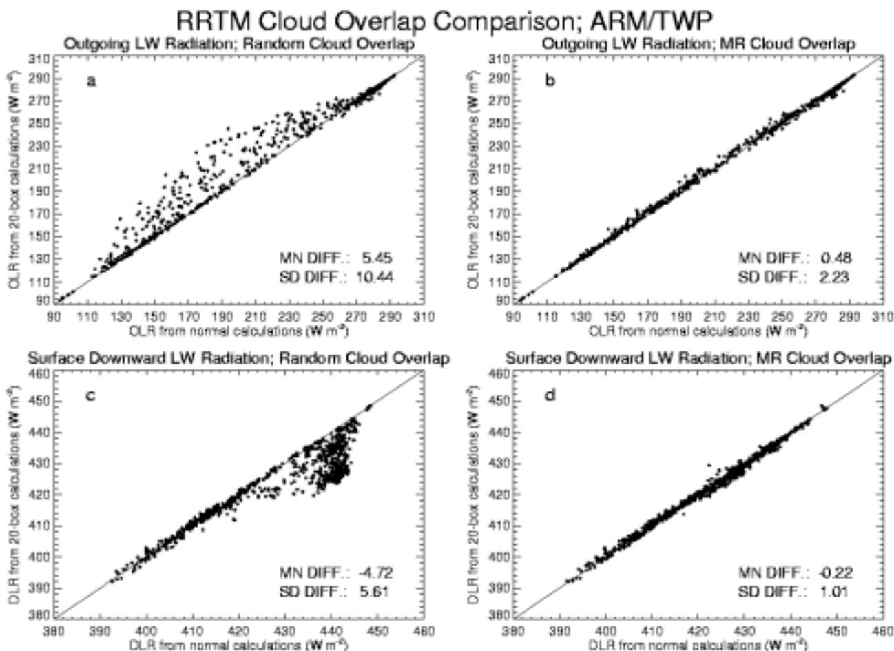
**Figure 1.** Scatter plot that compares RRTM longwave fluxes from a normal single-column calculation to a reference calculation using 20 sub-grid points (see text), for more than 700 ARM/TWP July 1997 profiles. Comparisons are shown for (a) OLR for random cloud overlap, (b) OLR for MR cloud overlap, (c) downward surface flux (DLR) for random overlap, and (d) DLR for MR overlap. The mean difference and standard deviation of the differences are also shown for each plot.
