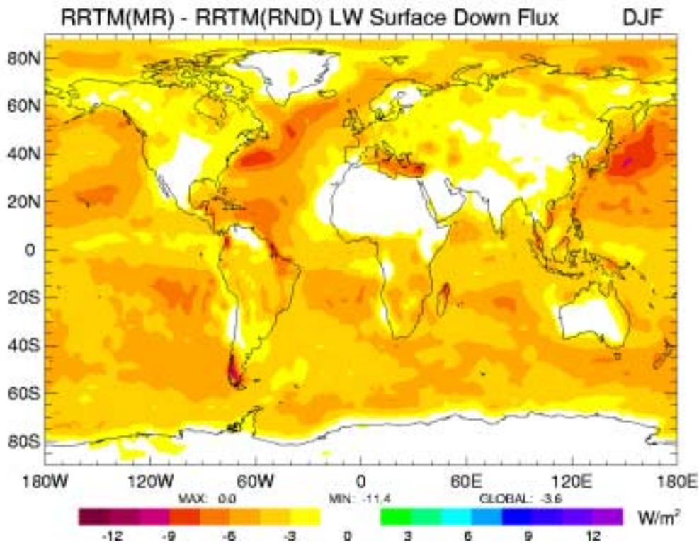
**Figure 3.** Initial forcing impact on downward longwave surface flux for Northern Hemisphere winter of maximum-random cloud overlap relative to random cloud overlap. Difference is between two parallel RRTM longwave calculations using each overlap method within a CCM3 simulation that used climatological sea surface temperatures.
