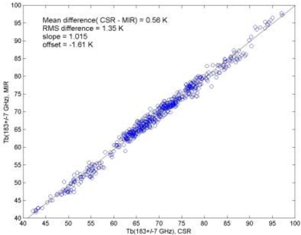
**Figure 2.** Statistics of comparisons between CSR and MIR  $183.31 \pm 7$  channels. Data were collected during the experiment from March 7 to March 30, 1999. Each data point is a 10-min average.
