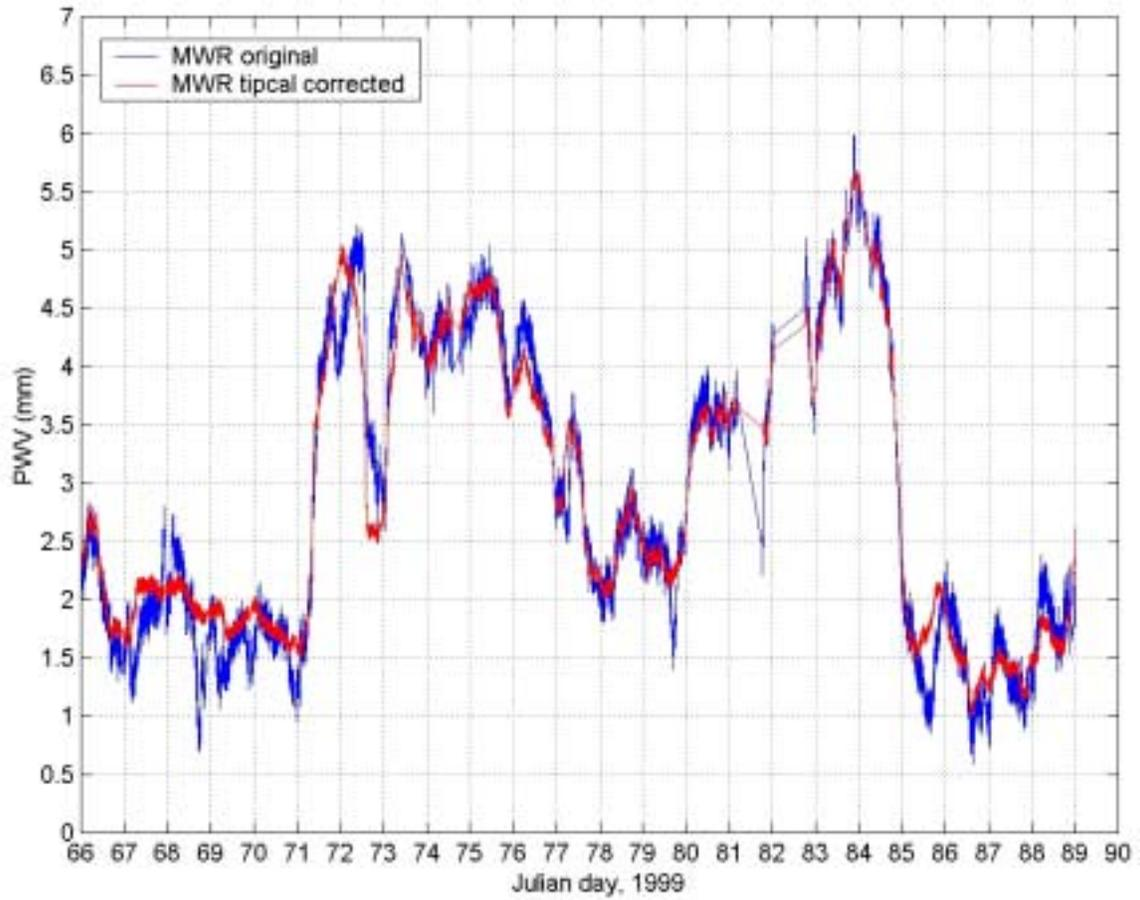
**Figure 5.** Time series of PWV obtained from the ARM-archived MWR data file and derived from the MWR measurements that are recalibrated at ETL using instantaneous calibration factors.
