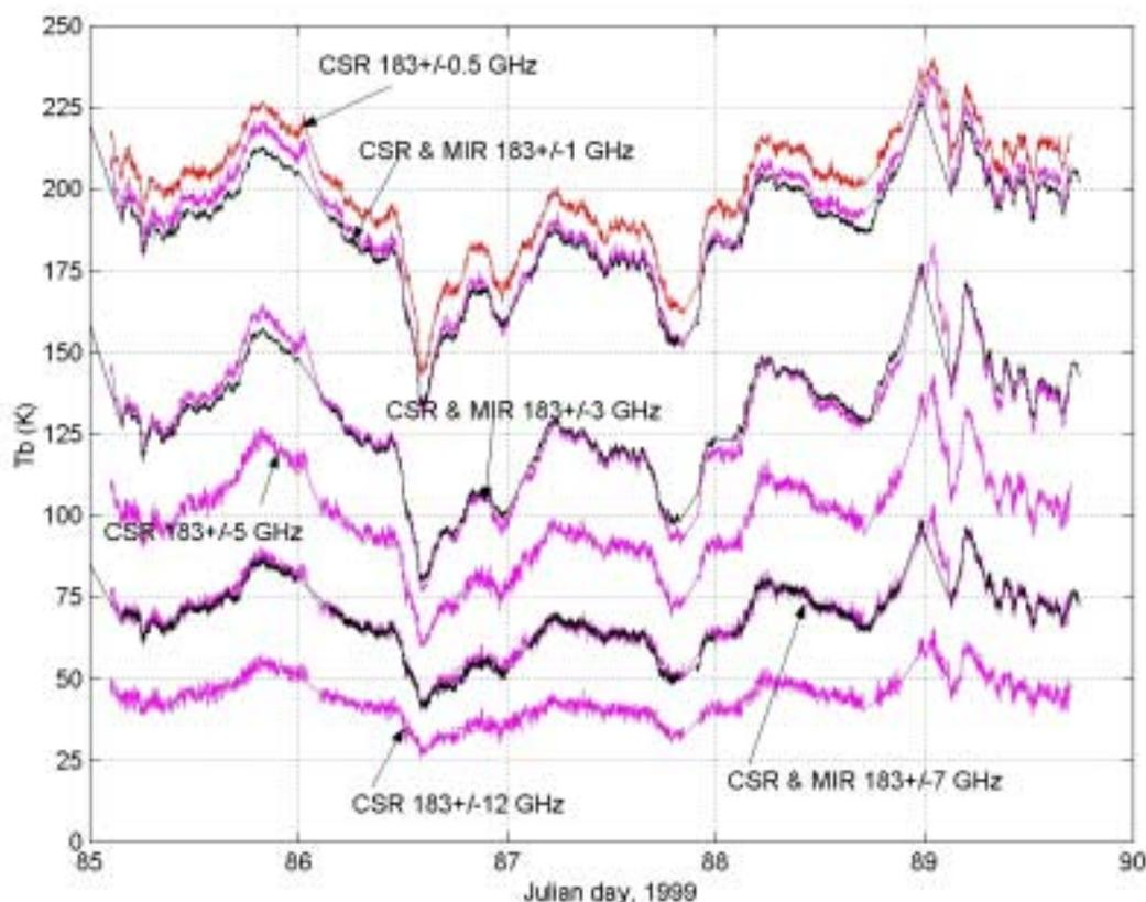
**Figure 1.** Time series of  $T_b$  around 183 GHz. Red line - CSR; black line - MIR. The CSR channels were calibrated using the tipcal procedure and the MIR channels were calibrated with two external blackbody references.
