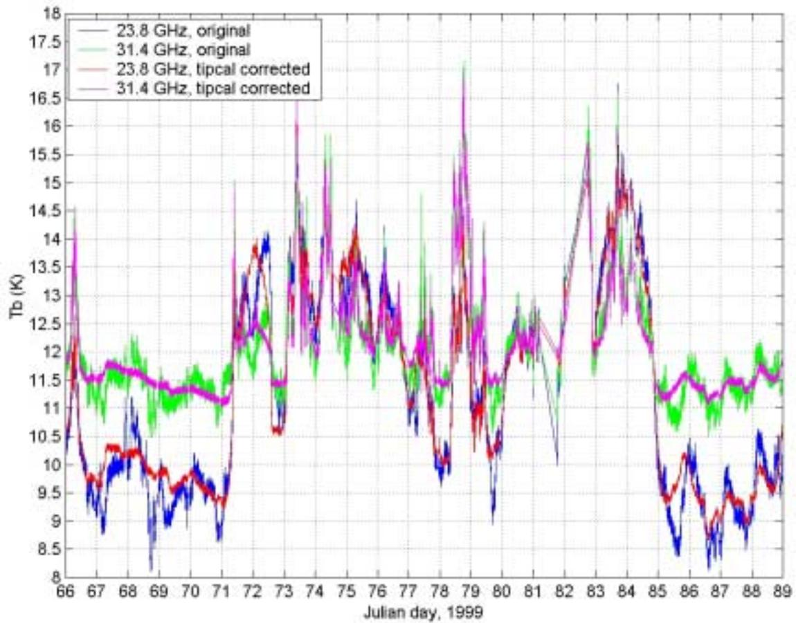
**Figure 3.** Comparisons of MWR  $T_b$  measurements. The green and blue lines are measurements obtained from ARM-archived MWR data files. These measurements were calibrated with a tipcal method in which the calibration factors are averaged over a specified period. The magenta and red lines are measurements that were recalibrated by ETL using instantaneous calibration factors.
