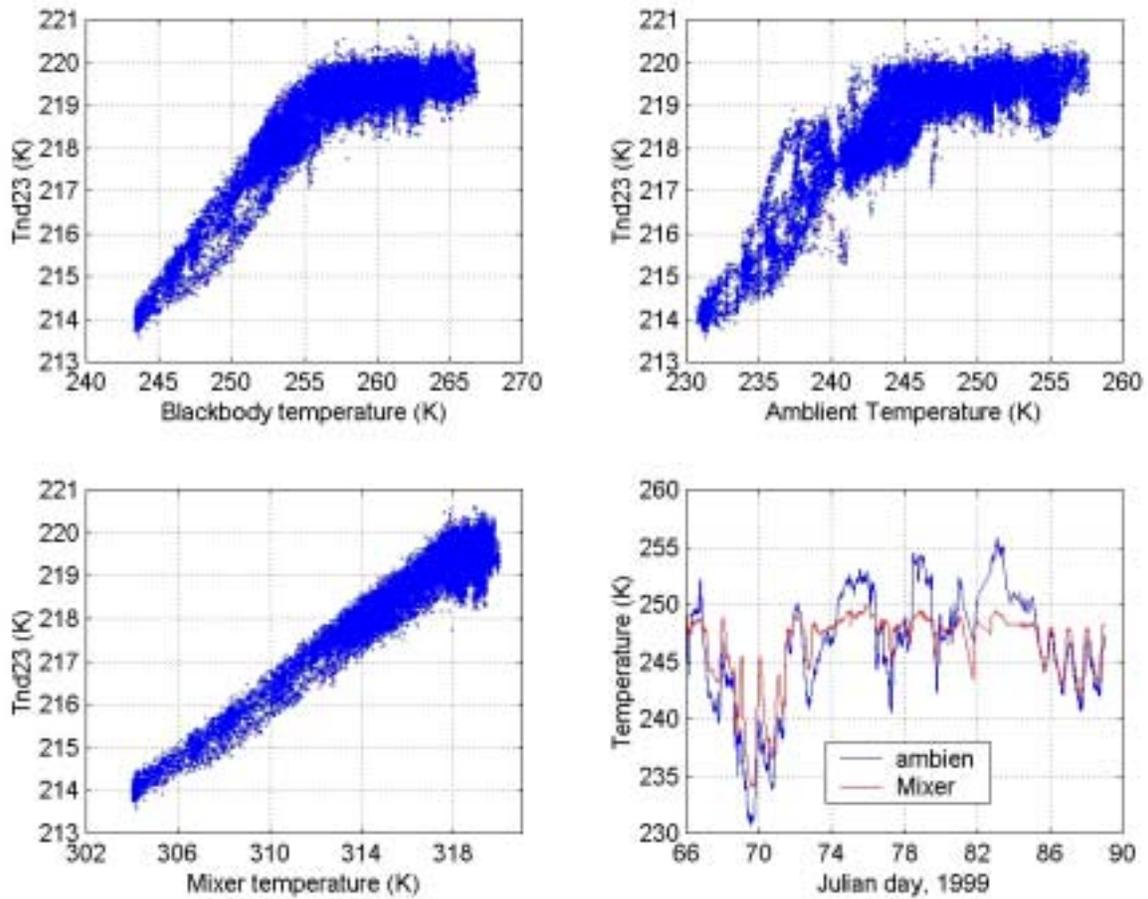
**Figure 4.** A: Tnd versus blackbody reference temperature. B: Tnd versus ambient temperature. C: Tnd versus mixer temperature. D: Time series of ambient and mixer temperatures.
