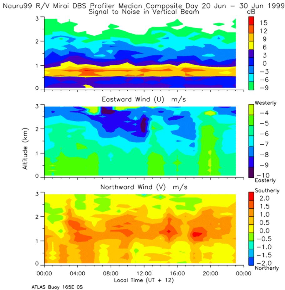
Figure 5. Wind profiler composite day, signal to noise, and eastward and northward wind components.
