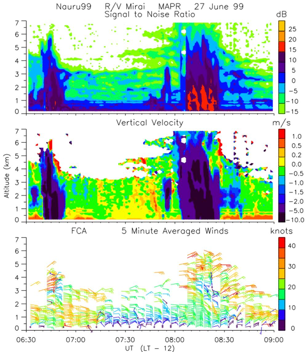
**Figure 3.** MAPR observations of two squalls from the deck of the R/V Mirai at 165°E, 0°S.
