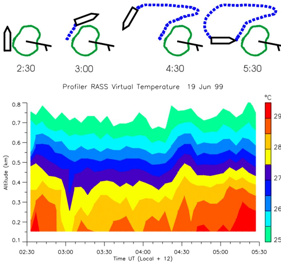
**Figure 2.** Island heating observations with RASS. The schematic maps indicate the course of the R/V Mirai with respect to Nauru island (green) at the indicated times, the wind barbs indicate the average wind. The contour plot shows the RASS virtual temperature from the deck of the Mirai.
