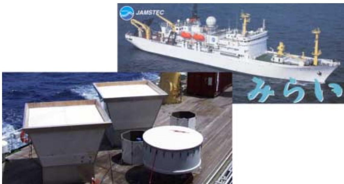
**Figure 1.** The R/V Mirai and radars on the aft deck. The two UHF profilers are in the large white boxes, which make up the clutter screens and stabilization platforms; MAPR is the profiler in the foreground; the DBS profiler is behind MAPR and is surrounded by four RASS speakers. The drum antenna is the NOAA/ETL S-band radar.
