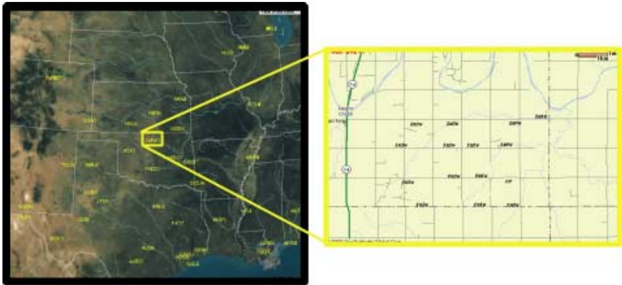
Figure 1. The NOAA-FSL and CORS sites are shown in the large view of the central United States. The single-frequency GPS systems are deployed around the ARM Central Facility. Each station in the single-frequency network is placed within an 8 km x 8 km rectangular grid. The spacing between each station is approximately 2 km.
