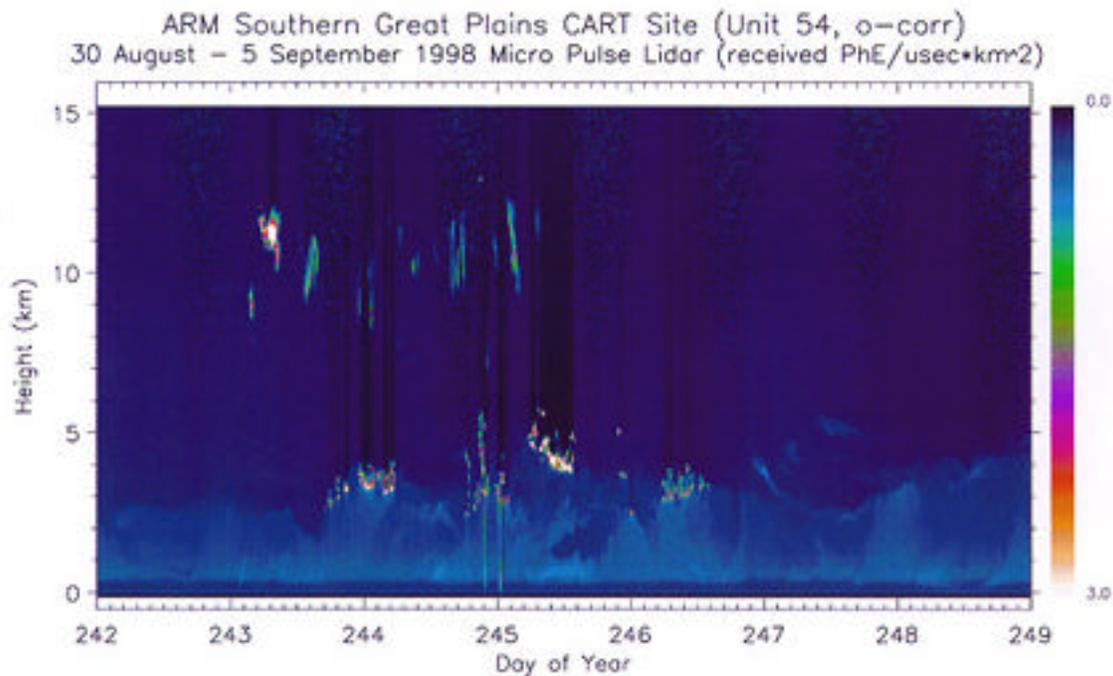
**Figure 2.** Overlap corrected returned raw backscatter counts from the SGP CART MPL for the week August 30 through September 5.
