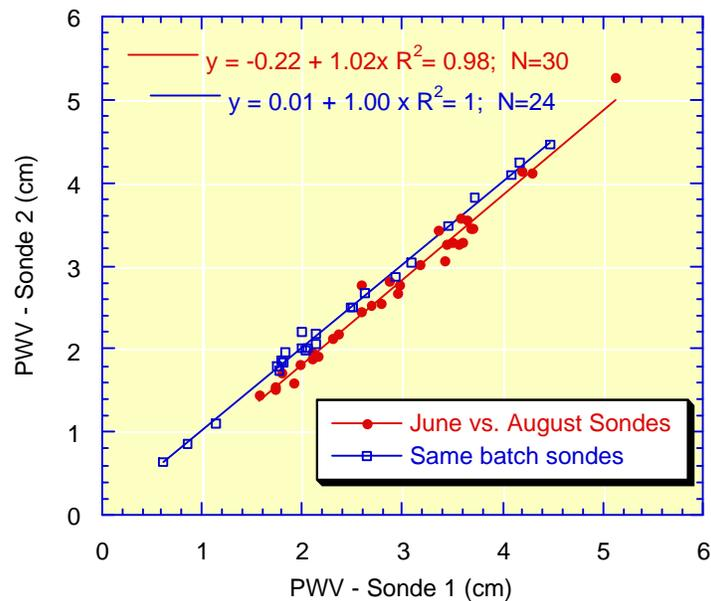
**Figure 5.** Comparison of uncorrected integrated PWV measured by dual-sonde soundings during the 1996 WVIOP. Results are grouped by calibration batch type (mixed or same).
