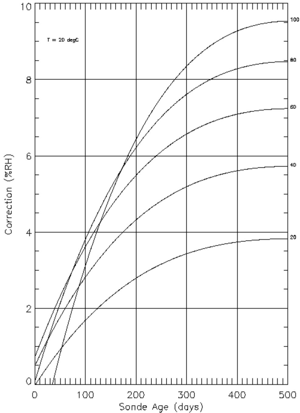
**Figure 10.** Total correction calculated for an ambient temperature of 20 °C for a range of RH values as a function of radiosonde age. The correction increases rapidly with sonde age and approaches a constant value beyond an age of 1.5 years.
