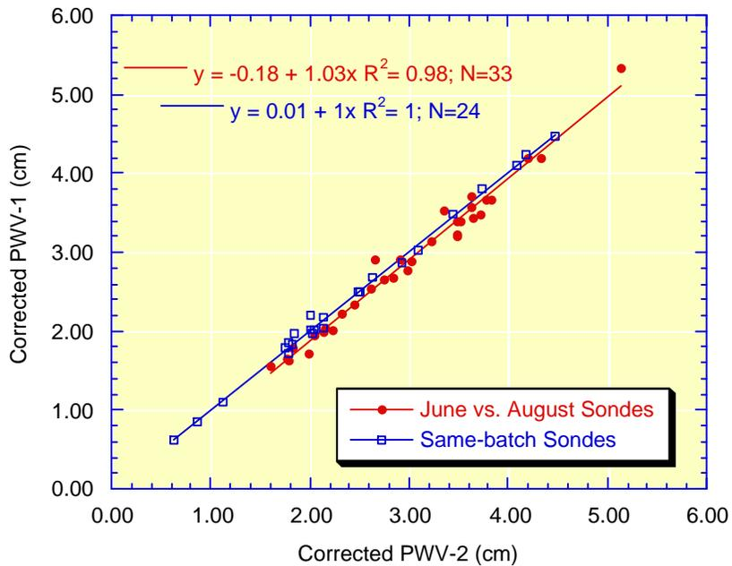
**Figure 7.** Comparison of integrated PWV measured by dual-sonde soundings during the 1996 WVIOP after the Vaisala correction is applied. Compare with Figure 5.
