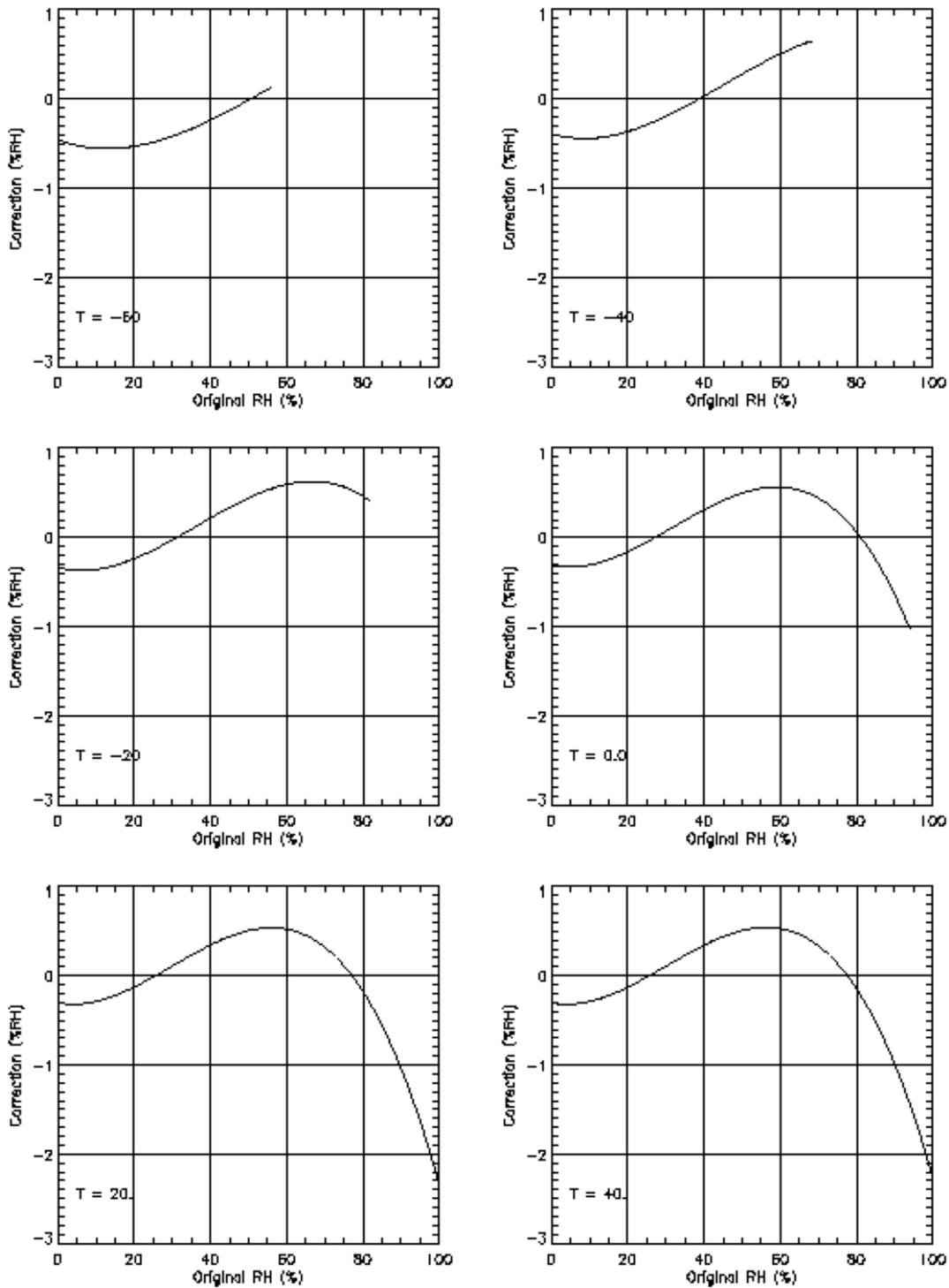
**Figure 1.** Correction factor to account for errors in the accuracy of the basic RS-80H calibration model. The correction depends on temperature and relative humidity (RH) and is shown to the approximate limit of saturation with respect to water for each temperature panel.
