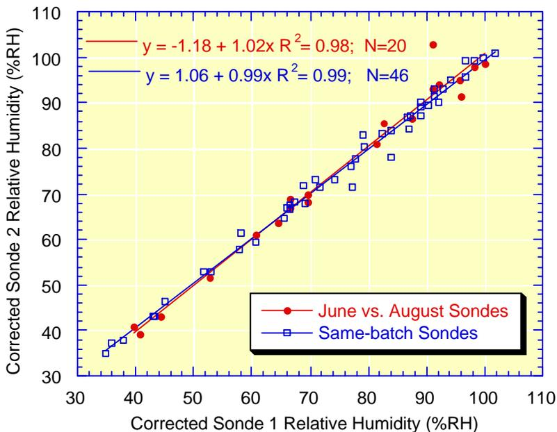
**Figure 9.** Comparison of surface RH measured by dual-sonde soundings during the 1997 WVIOP after the Vaisala correction is applied. Compare with Figure 8.
