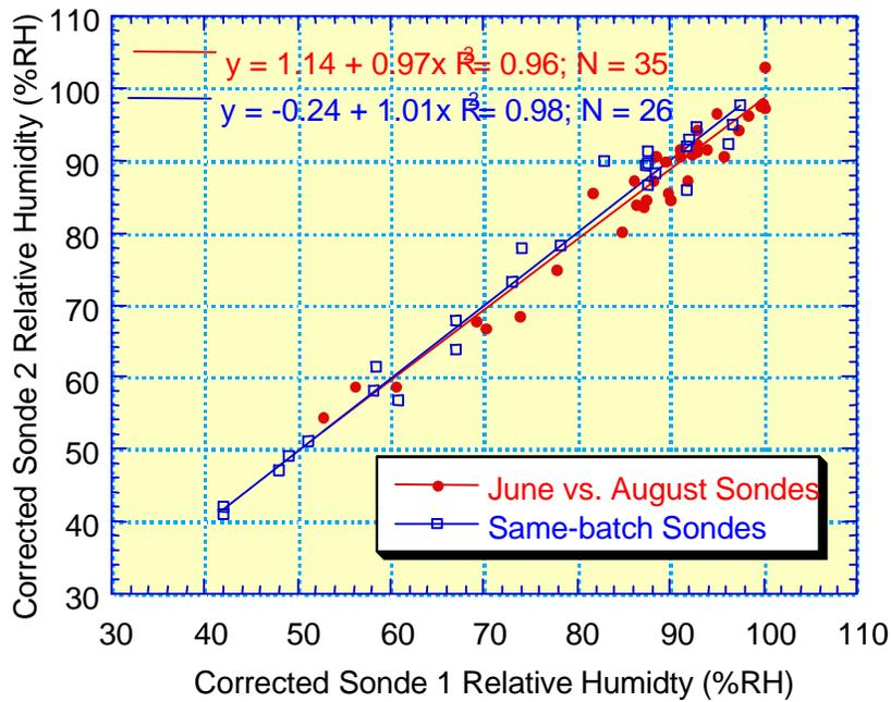
**Figure 6.** Comparison of surface RH measured by dual-sonde soundings during the 1996 WVIOP after the Vaisala correction is applied. Compare with Figure 4.
