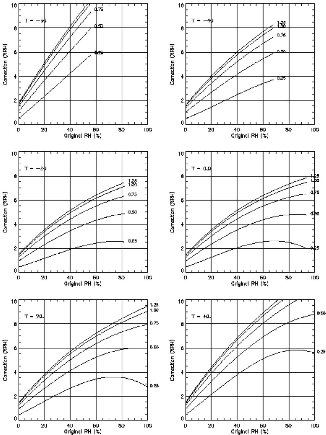
**Figure 3.** The total correction applied to the RS-80H humidity sensor. The total correction includes the calibration model and bias corrections (Figures 1 and 2) as well as an additional minor correction (not shown) related to the accuracy of the RS-80H humidity sensor at low-temperature saturation. As in Figure 2, the curve families in each panel are for radiosondes of ages between 0.25 and 1.25 years.
