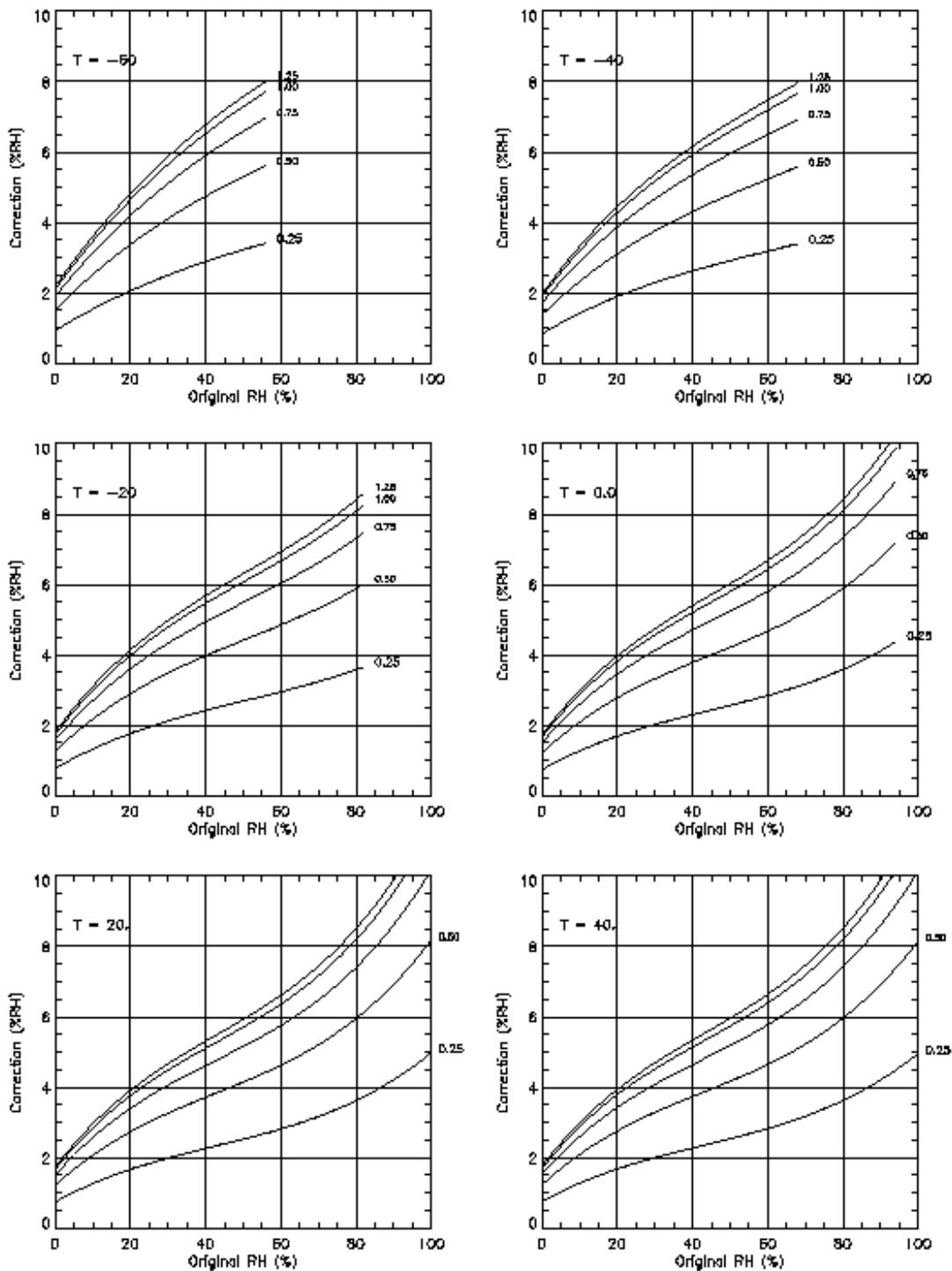
**Figure 2.** Correction factor to account for dry bias caused by contamination of the RS-80H humidity sensor. The correction depends on temperature, RH, and radiosonde age (curve families). The corrections are shown to the approximate limit of saturation with respect to water for each temperature panel.
