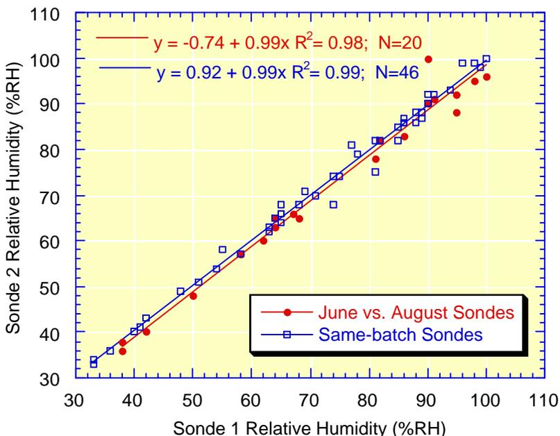
**Figure 8.** Comparison of uncorrected surface RH measured by dual-sonde soundings during the 1997 WVIOP.
