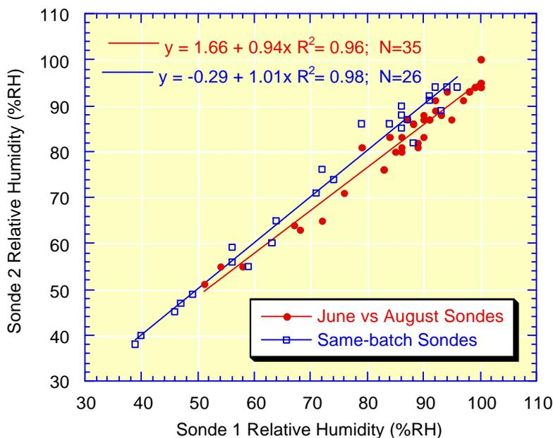
**Figure 4.** Comparison of uncorrected surface RH measured by dual-sonde soundings during the 1996 WVIOP. Results are grouped by calibration batch type (mixed or same).
