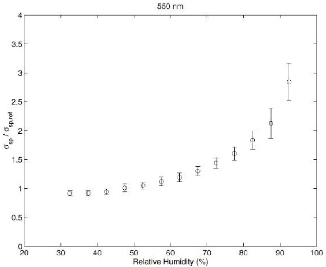
**Figure 1.** The ratio of the scattering coefficient measured under wet conditions to that measured under dry conditions as a function of the RH of wet conditions for the three wavelengths. The relation is obtained by fitting second order polynomials to data. Open circles and error bars indicate averaged values and standard deviations for every 5% RH intervals.
