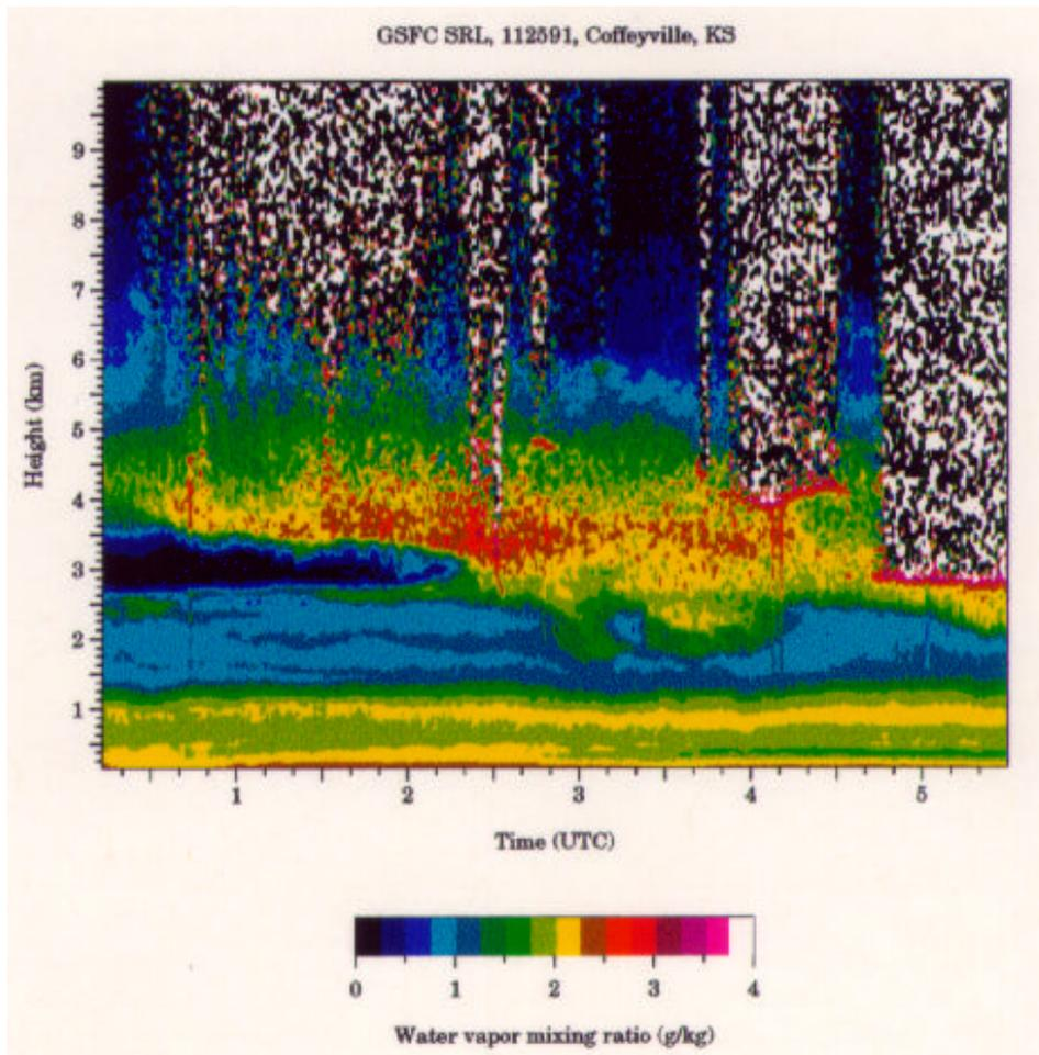
**Figure 4.** SRL-sensed water vapor mixing ratio ( $\text{g kg}^{-1}$ ) profiles on November 25, 1991, over Coffeyville, Kansas. Note the vertical stipling, which indicates attenuation by cloud.
