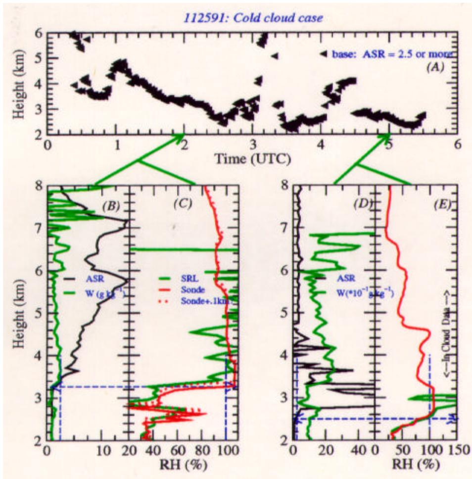
**Figure 3.** Time series of SRL-derived CBH (a), and profiles of SRL data at 0200 UTC (b) and 0500 UTC (d) showing ASR (black) and water vapor (green). Sonda (red) and SRL (black) measured profiles of RH (red) and at 0200 UTC (c) and 0500 UTC (e) are also compared.
