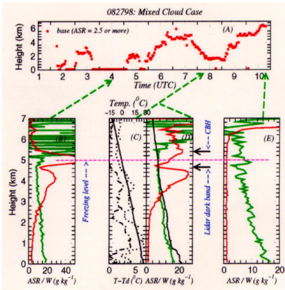
**Figure 2.** Time series of CBH (a), ASR (black) and W (green) profiles at three selected times: 0400 UTC (b), 0745 UTC (d) and 1020 UTC (e) and sonde profiles (c) of temperature (red) and both the “corrected” and uncorrected (dotted) dewpoint depression (violet) profiles are shown. The sonde derived mixing ratio (black) is also shown in (c) for comparison.
