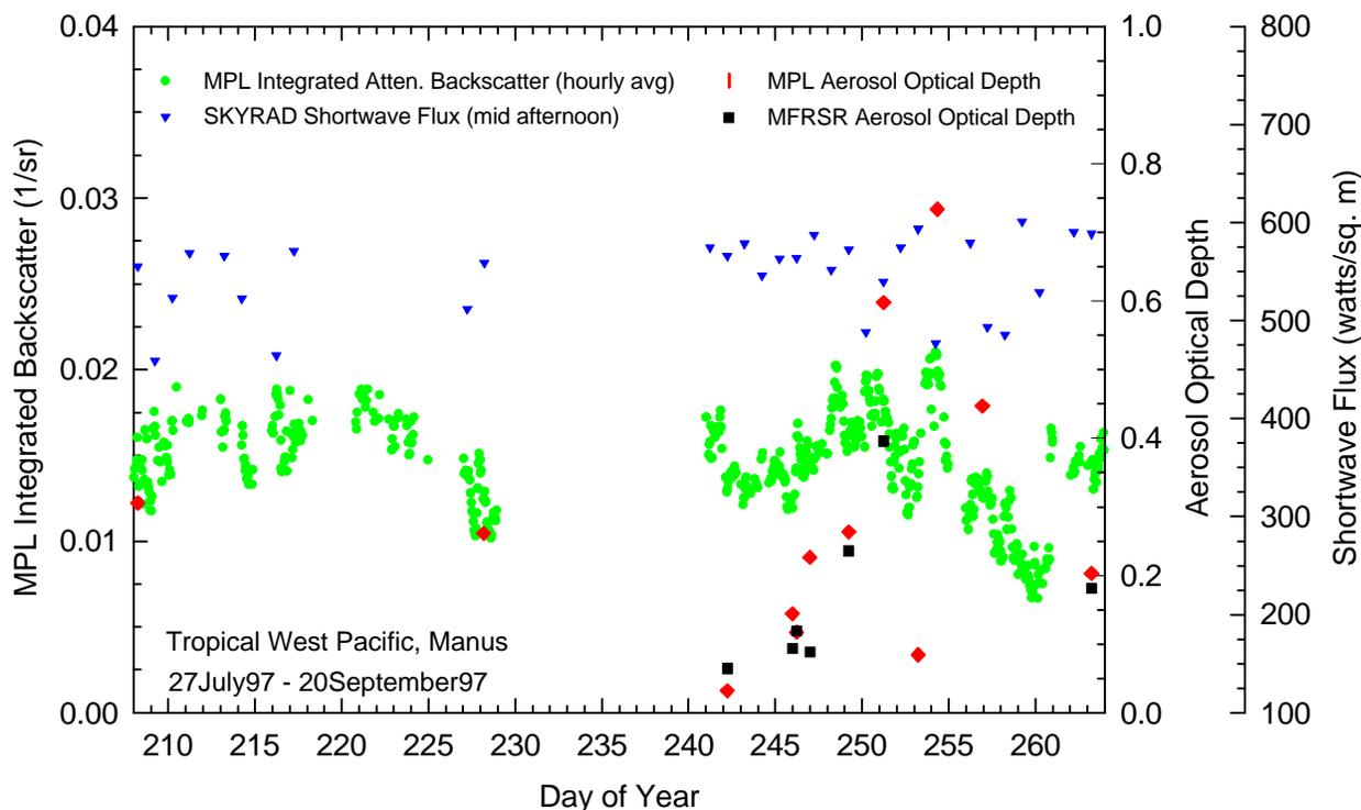
**Figure 3.** Cloud-cleared optical and radiation measurements at the TWP site from July to September 1997. (For a color version of this figure, please see [http://www.arm.gov/docs/documents/technical/conf\\_9803/spinirne-98.pdf](http://www.arm.gov/docs/documents/technical/conf_9803/spinirne-98.pdf).)
