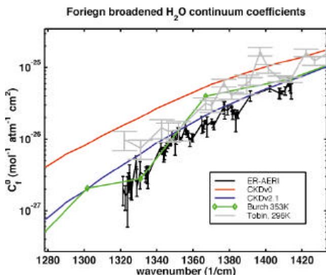
**Figure 2.** AERI-derived continuum values compared with laboratory measurements. (For a color version of this figure, please see [http://www.arm.gov/docs/documents/technical/conf\\_9803/knuteson-98.pdf](http://www.arm.gov/docs/documents/technical/conf_9803/knuteson-98.pdf).)
