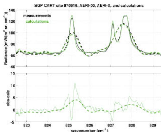
**Figure 3.** Using AERI (medium resolution) and AERI-X (high resolution) to evaluate infrared H<sub>2</sub>O line strength and width accuracy. (For a color version of this figure, please see [http://www.arm.gov/docs/documents/technical/conf\\_9803/knuteson-98.pdf](http://www.arm.gov/docs/documents/technical/conf_9803/knuteson-98.pdf).)
