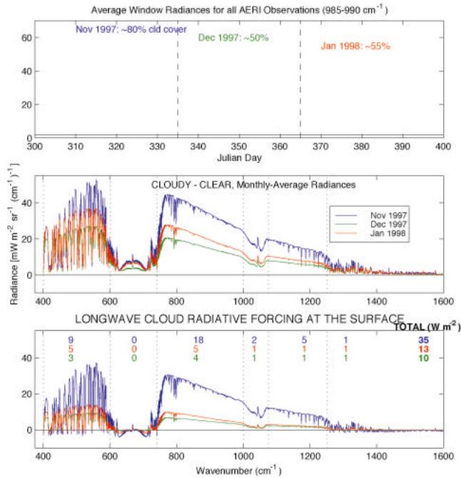
**Figure 5.** Preliminary estimates of cloud radiative forcing from AERI-ER observations. The rows of numbers in the lower panel (top to bottom) correspond to the cloud radiative forcing for November 1997, December 1997, and January 1998. (For a color version of this figure, please see [http://www.arm.gov/docs/documents/technical/conf\\_9803/knuteson-98.pdf](http://www.arm.gov/docs/documents/technical/conf_9803/knuteson-98.pdf).)
