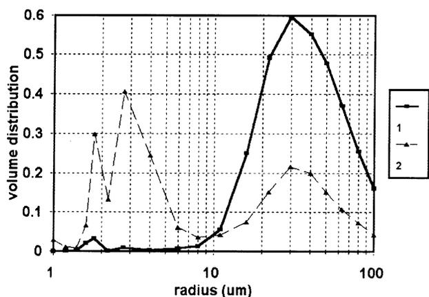
**Figure 3.** Volume size distributions retrieved from MWMFOV measurements at Zvenigorod. 1 - Ci, 28.07.97; 2 - Ci + Cu, 30.07.97.
