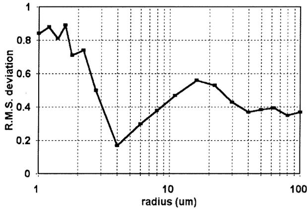
Figure 1. Rms estimation of the cloud particle size.
