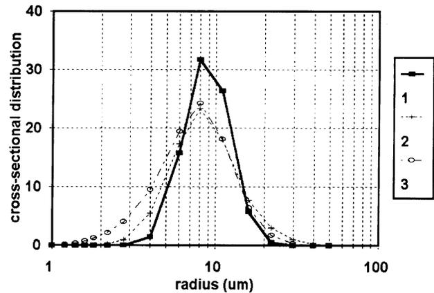
Figure 2. Inversion of the MWMFOV data set for the model size distribution. 1 - initial lognormal; 2 - inverted; 3 - inversion with input parameters disturbed by 3% random error.
