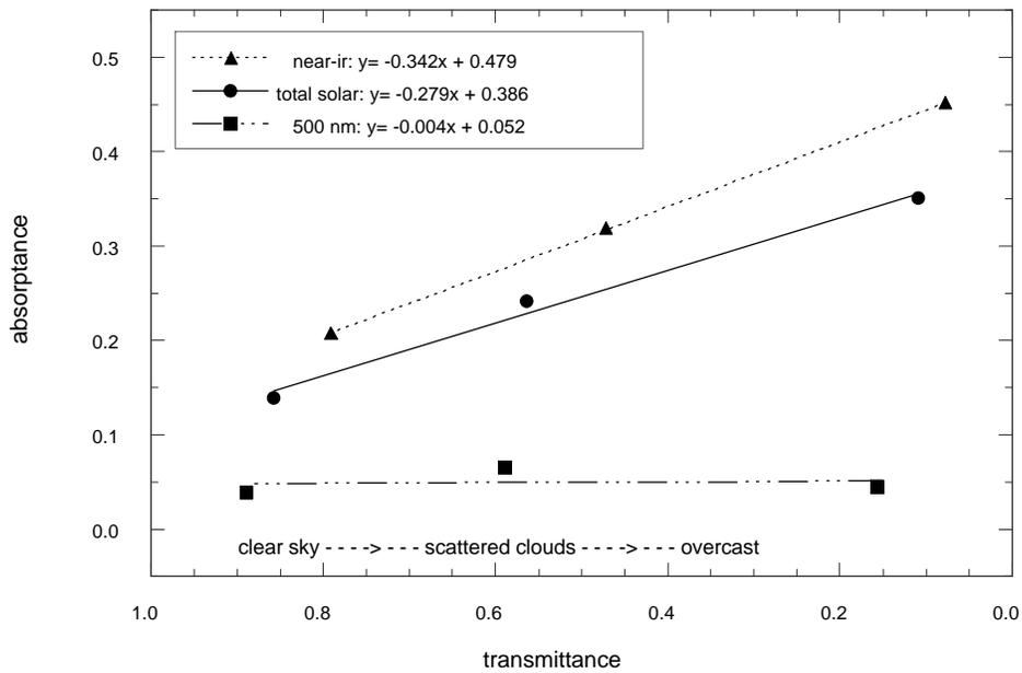
**Figure 2.** Column absorbance as a function of column transmittance (as defined in text) for each of three bandpasses as labeled.
