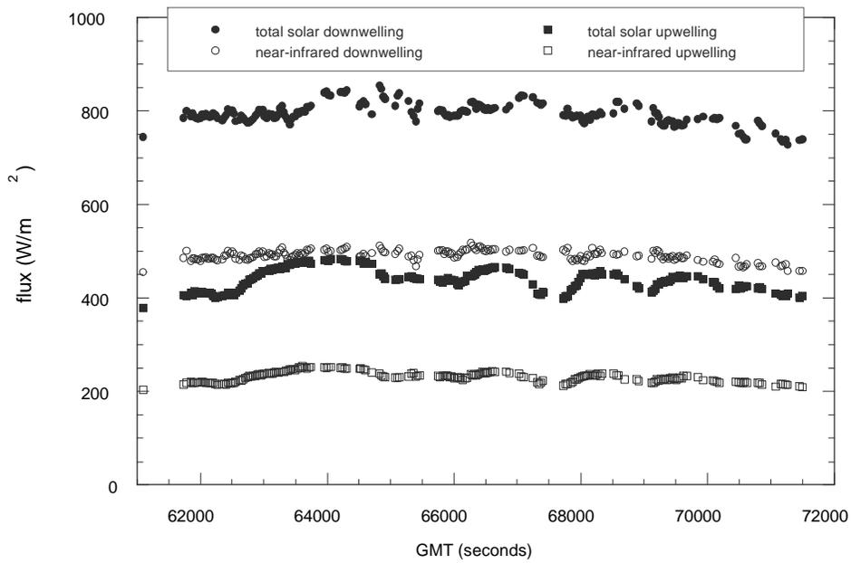
**Figure 1.** Broadband fluxes as a function of time, measured at 13 km altitude on October 30, 1995
