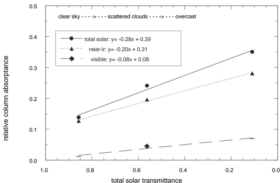
**Figure 3.** Relative column absorptance vs. total solar transmittance, for the total solar bandpass and its near-infrared and visible halves.
