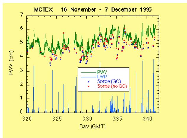
**Figure 1.** Time series of integrated or “precipitable” water vapor (PWV) and liquid water path (LWP) from the microwave radiometer. Periods of precipitation have been eliminated. The circles are PWV derived by integrating radiosonde soundings, with and without the effect of the calibration ground check. (See text for explanation of the ground check.)
