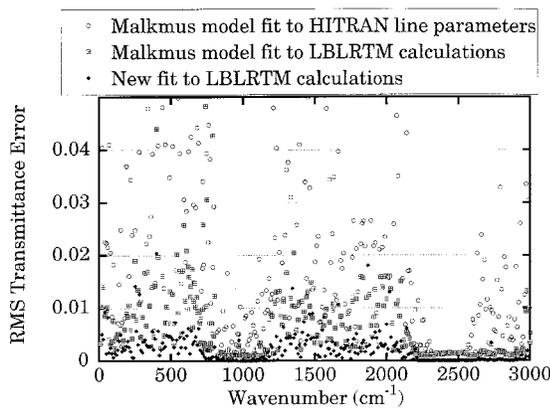
**Figure 2.** Spectral distribution of RMS transmittances differences between band models and LBLRTM.
