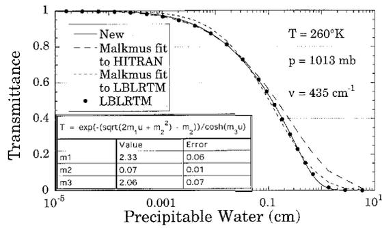
**Figure 1.** An example of the least squares fit of transmittances to LBLRTM calculations.
