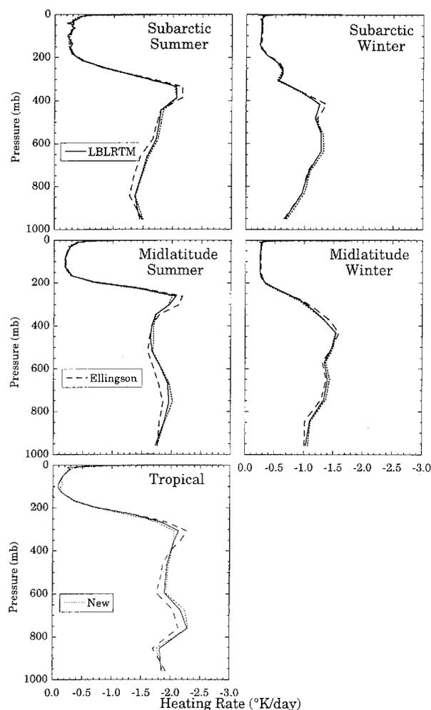
**Figure 3.** Heating rates calculated from water vapor line absorption only (no continuum) for McClatchey standard atmospheres.
