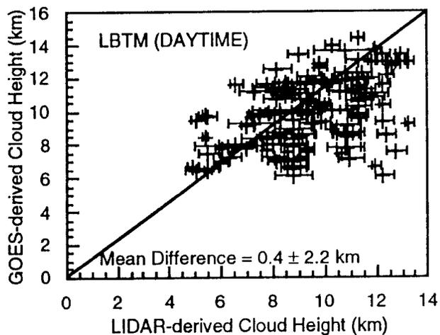
**Figure 4.** Comparison of high thin cloud heights derived from GOES with MPL cloud height estimates.
