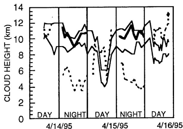
Figure 2. Cloud heights over the SCF. Lidar-derived cloud boundaries are thin solid lines; satellite-derived cloud heights are dashed (LBTM during the day, IRONLY at night) and thick solid (3-channel method) lines.
