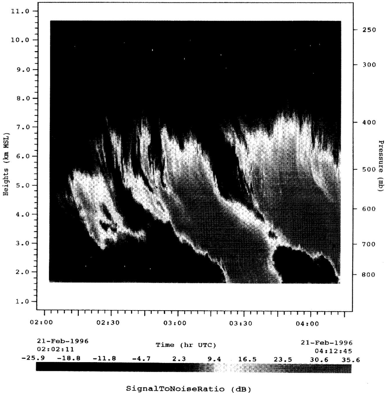
**Figure 4.** Convective clouds observed at the Erie site February 21, 1996, from 2:00 to 4:00 UTC. Light precipitation was measured at the surface at 3:30 UTC. The radar was operated with low power. Range resolution is 45 m with a 20-sec sampling interval.
