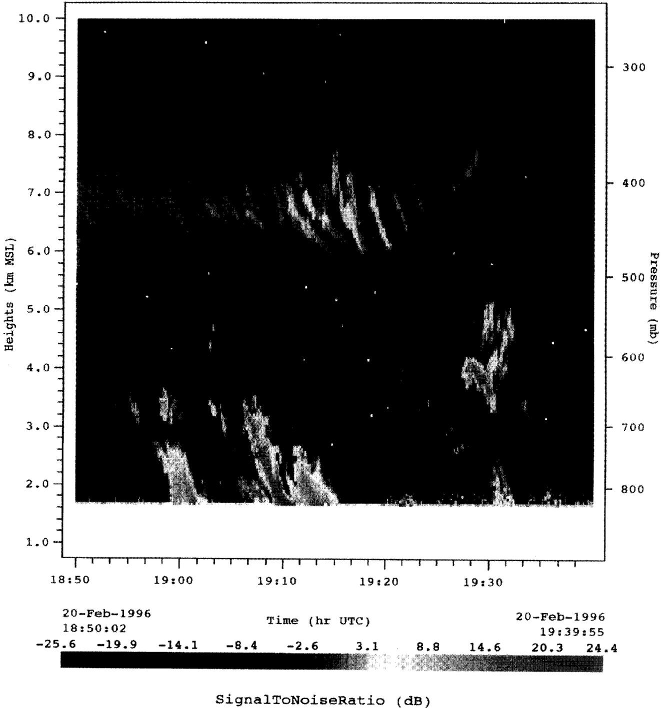
**Figure 3.** Wave-like structure observed at 7 km on February 20, 1996, 19:20 UTC at Erie, Colorado. This field site is located near the front range of the Rocky Mountains and wave patterns are often observed. Range resolution is 45 m with 10-sec averaging time.
