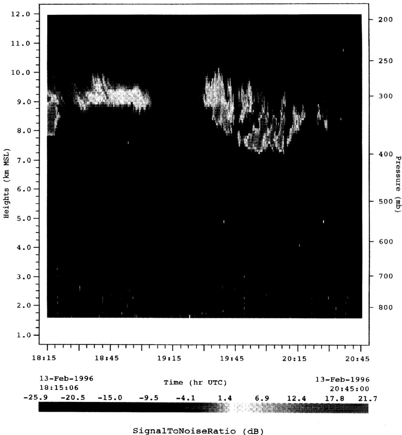
**Figure 2.** Cirrus clouds observed from 18:00 to 21:00 UTC February 13, 1996, at Erie, Colorado. The cloud's backscattered power is displayed in terms of S/N (an uncalibrated measurement). Range resolution is 90 m with 10-sec averaging time.
